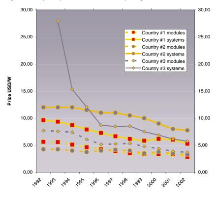
Figure 5 shows a continuing downward trend in grid-connected system prices in selected countries and the associated less-variable downward trend for the module prices. The convergence of prices in the different countries continues, indicating the worldwide trading of modules and the attention to some of the non-technical barriers.
