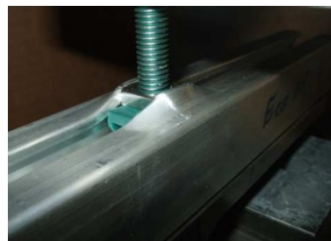
Fig. 15: Screw canal bends due to mechanical stress [19].
