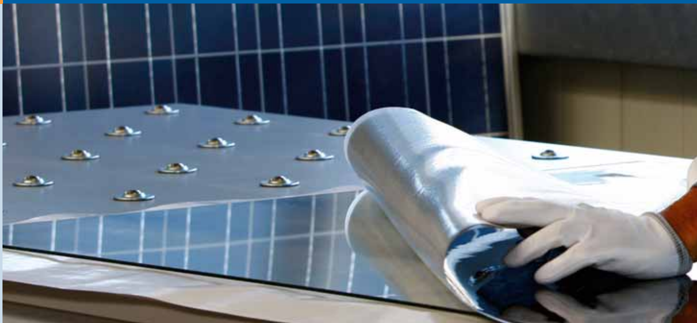
Fig. 2 - Development of composite films for encapsulating photovoltaic modules (photo: Isovolta).
