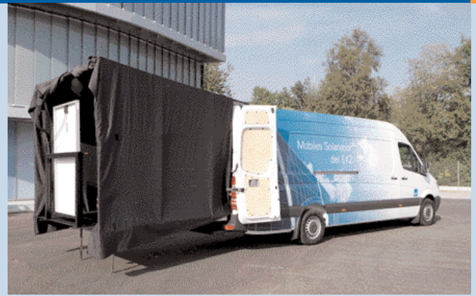
Fig. 3 - Mobile test equipment. With the support of the utility of the Canton of Zurich, the University of Applied Sciences in Winterthur has built a mobile test unit which allows PV module testing at the site of a PV plant (photo EKZ, Zurich).
