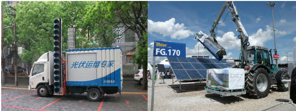
Fig. 1.1-15 Cleaning by specific water vehicles
