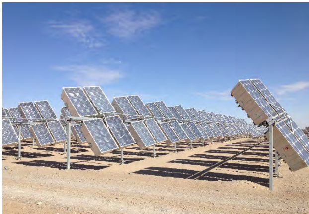
Fig. 1.1-12 Simplest Bearing-Free Turning System by SunCore, Qinghai, China
