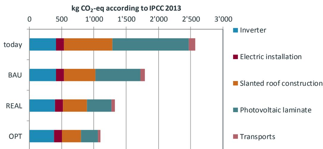
Fig. 6.2 Greenhouse gas emissions of CdTe-based 3-kWp photovoltaic power plants installed on slanted roofs in Europe according to the three scenarios (BAU, REAL and OPT) in kg CO<sub>2</sub>-eq (according to IPCC (2013), Tab. 8.A.1, 100a) showing the contribution of the different parts.
