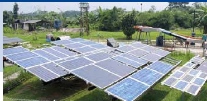
Fig. 3 - PV module reliability test site in Indonesia studying the stress factors of PV modules failures under real time outdoor testing compared to accelerated stress conditions (Photo: TÜV Rheinland).
