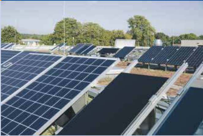
Fig. 3 – Outdoor PV module efficiency and energy yield test facility (Photo: © Fraunhofer CSP, Halle).
