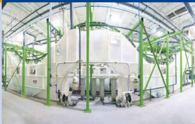
Fig. 1 – The latest generation, continuous processing reactor for the recycling of thin film solar panels at First Solar, Perrysburg Ohio, USA. PVPS Task 12 Experts visited this facility in September 2016.
