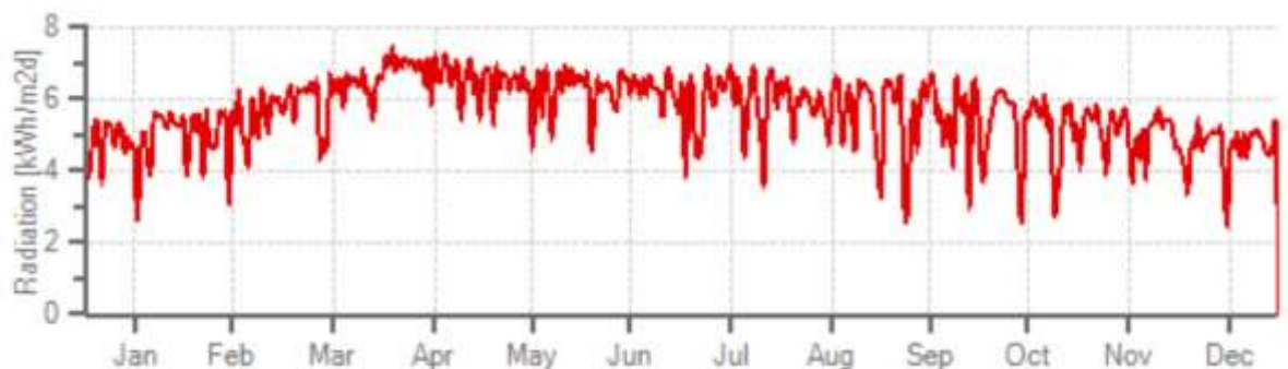
Figure 21: The horizontal solar irradiation of the site
