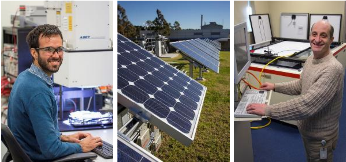
Figure 6: CSIRO's PV Performance Laboratory consists of NATA accredited cell testing, advanced outdoor testing and calibrated module flash testing. (CSIRO, 2015)
