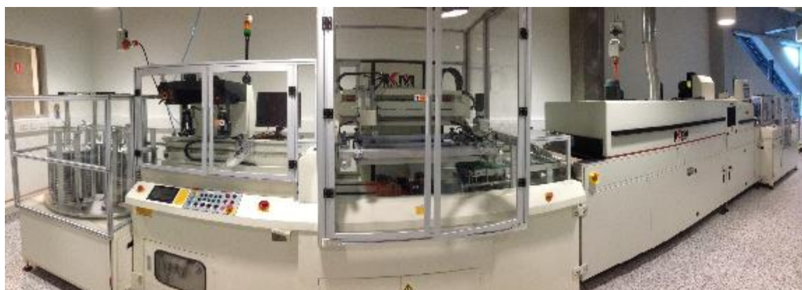
Figure 10: Screen printing line for printing dye sensitised solar cells. (Monash University, 2015)
