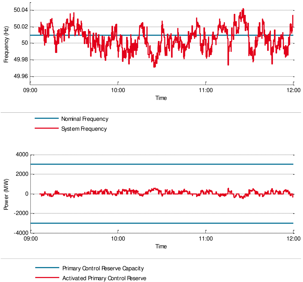
Figure 5: Progression of the self-measured net frequency and resulting activation of primary control reserve power. Data Source: Fraunhofer IWES.
