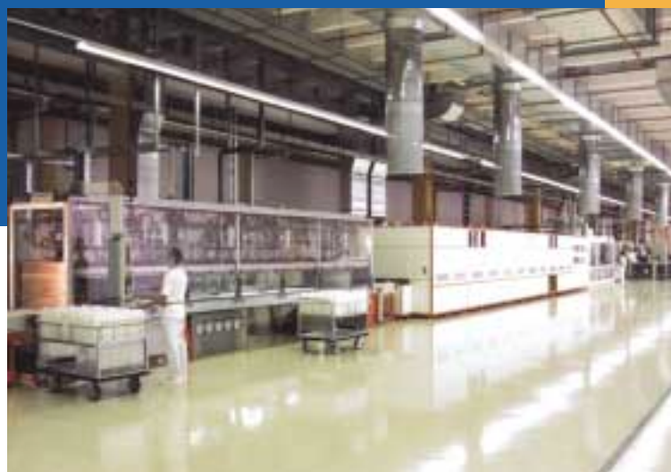
Fig. 2 – EFG Cell Production Line of RWE Schott Solar's SmartSolarFab™. (Photo RWE Schott Solar GmbH, Alzenau)
