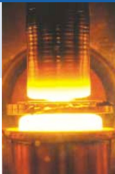
Fig. 3 - The Float-zone crystal growth process is used by Topsil Semiconductor Materials, for their specialised low-cost PV-FZTM wafer product dedicated the very high efficiency solar cell market.
