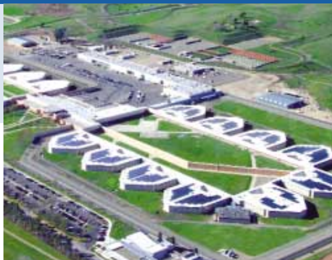
Fig. 3 - This 1,18 MW photovoltaic installation on the Santa Rita jail is located in Dublin, CA. It reduces peak power consumption by 30 % and produces over 1.4 million kWhr per year. (Photo Courtesy of PowerLight Corporation)
