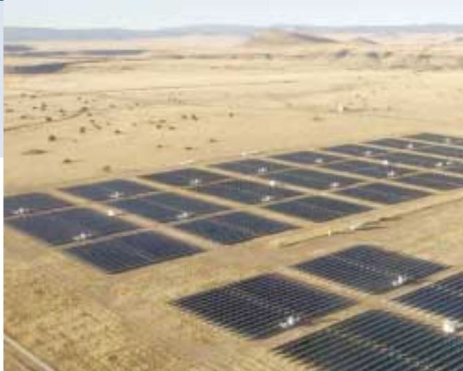
Fig. 3 - Tuscon Electric Power's Springerville Generating Station Solar System (SGSSS). 32,280 photovoltaic panels in eastern Arizona. The array currently produces more power than any single photovoltaic installation in the world, 4,958 mega-watt-hours (MWh) in 2003 and expected 6,400 MWh in 2004. (photo courtesy of Dave Sanders)
