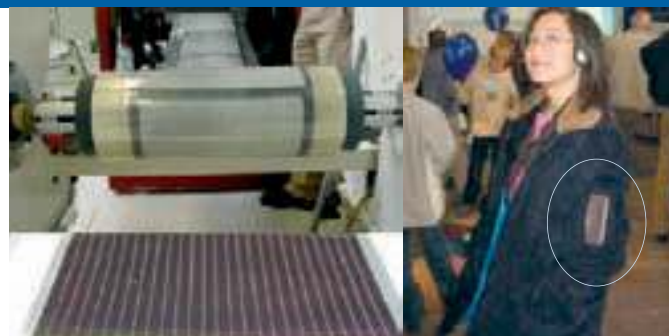
Fig. 1 - Successful roll-to-roll pilot line at AKZO (insert: coat mounted amorphous silicon thin film "module"), (photo AKZO Nobel Nederland).
