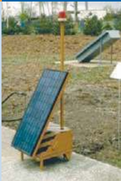
Fig. 6 - Photovoltaic Traffic Warning System of EIE.
