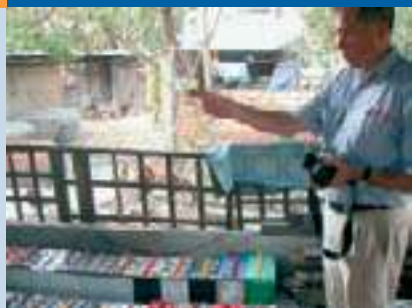
Fig. 2 - Car batteries are often charged at a central station (PV, hydro or diesel) and used in unelectrified homes for lighting and TV (Cambodia).
