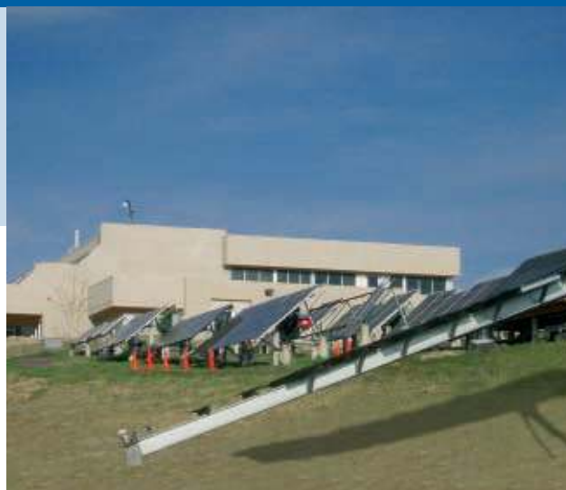
Fig. 3 - This view of NREL's Outdoor Test Facility shows the laboratory building and some of the test beds used to evaluate PV systems under field conditions.
