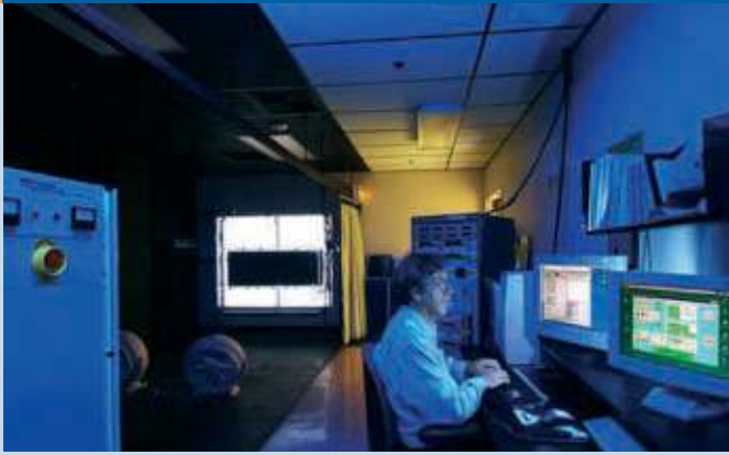
Fig. 1 - A researcher operates NREL's large area continuous solar simulator as part of the Measurements and Characterization activity.
