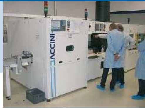
Fig. 2 – New technology at Solland Solar: laser edge insulation incorporated in the new 20 MW production line.
