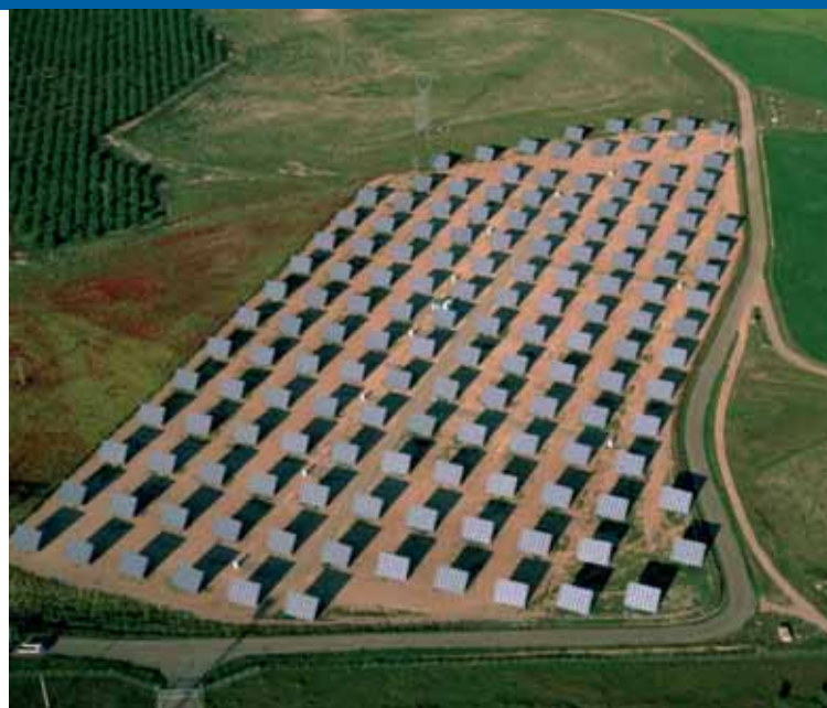
Fig. 1 - A 1,5 MW size grid-connected solar plant with different technology on the tracking system (photo courtesy of Tudela Solar, Navarra).
