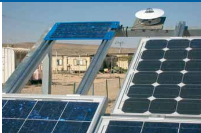
Fig. 1 - Part of a test stand at the BGNSEC, Sde-Boker, where module degradation is being quantified. The small PV panel (upper left) provides a trickle charge for batteries in a field data logger.
