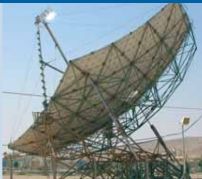
Fig. 2 - PETAL, the 400 m 2 solar dish at Sde-Boker, subjecting the HiConPV CPV module to 1 000X irradiance.
