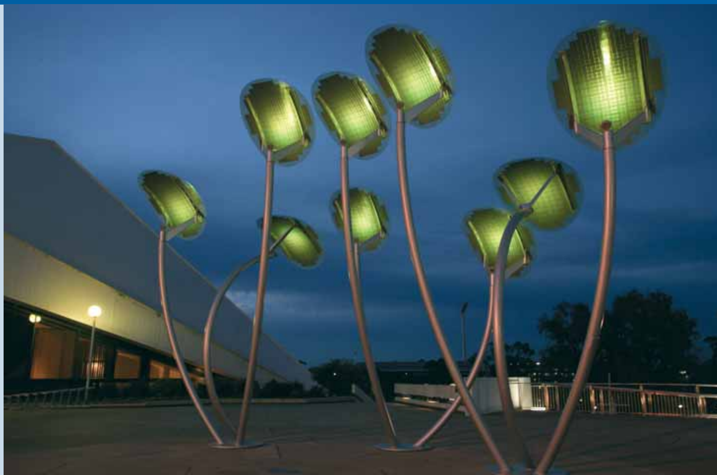
Fig. 1 - Solar Mallee Trees, Adelaide Festival Centre. Based on a design by the University of South Australia, individual solar cells were pieced together to form oval shaped solar panels. The panels are placed atop curved poles with the whole structure designed in the form of the indigenous mallee tree. There are 9 lights in total, 3 per mallee tree. The panels were formed by local company, Street Park and Furniture. The trees have an audio interpretative feature informing the public about Adelaide as a Green City. The original voices for this audio feature come from one of the City's first Solar Schools - Sturt Street Community School (photo Capital City Committee, a partnership between the South Australian Government and Adelaide City Council).
