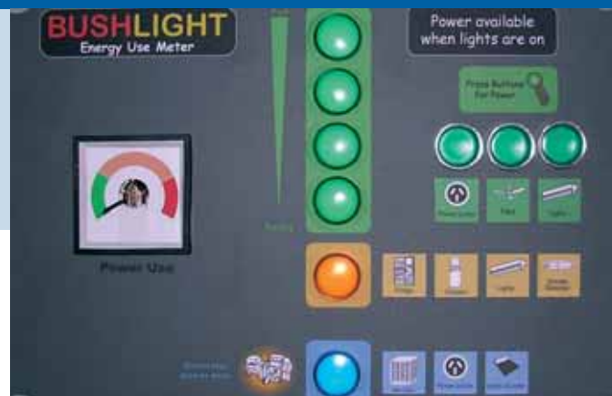
Fig. 2 – The Bushlight Energy Management Unit user interface.
