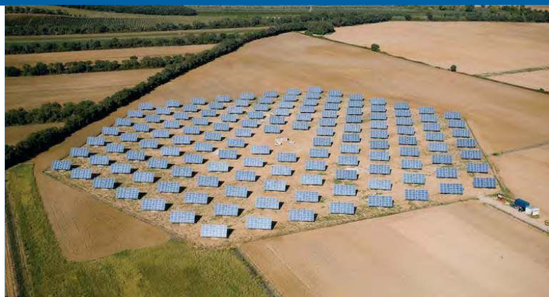
Fig. 1 - Sun tracking 1 MW PV plant, Roccastrada (GR) (photo GSE).
