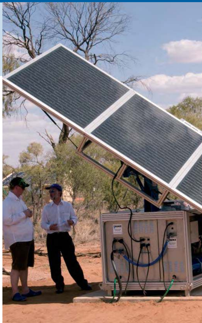
Fig. 3 – Tranz PV water pump at the Desert Springs Solar Test Centre, Alice Springs (photo Simon Troman).
