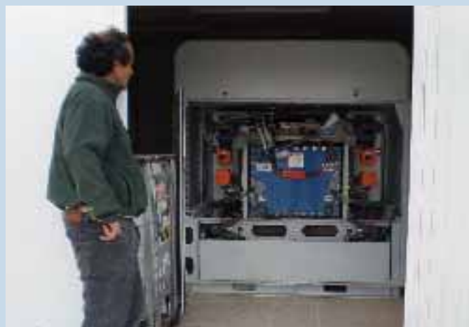
Fig. 4 - A 5 kW vanadium redox flow battery under study at Sde Boker for interfacing a PV array to the grid.
