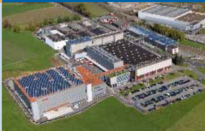
Fig. 2 - Edison Power 840 kW PV on 3 different roofs at the PISTOR facility in Rothenburg (photo: PISTOR).
