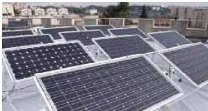
Fig. 2 - Bifacial modules outdoor test site at the Jerusalem College of Technology.
