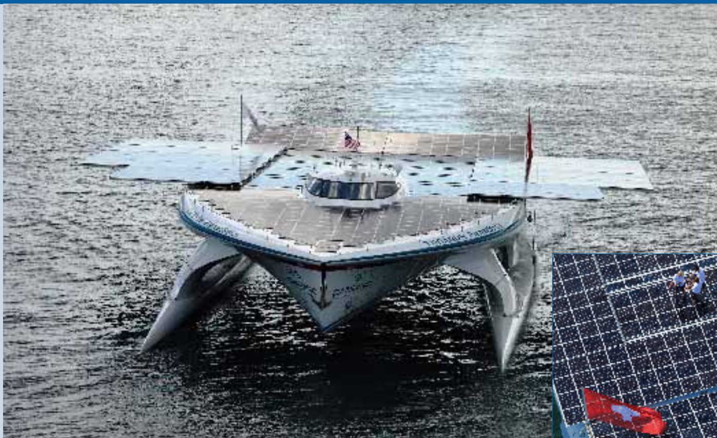
Fig. 1 - The PlanetSolar boat in Miami after crossing the Atlantic. The boat is 31 m long and 15 m wide; with further extensions it has space enough for more than 500 m 2 of solar panels with a total power of 93 kW. The energy is stored in 648 Li-ion batteries which give the boat an autonomy of about three days. (photo: © PlanetSolar).
