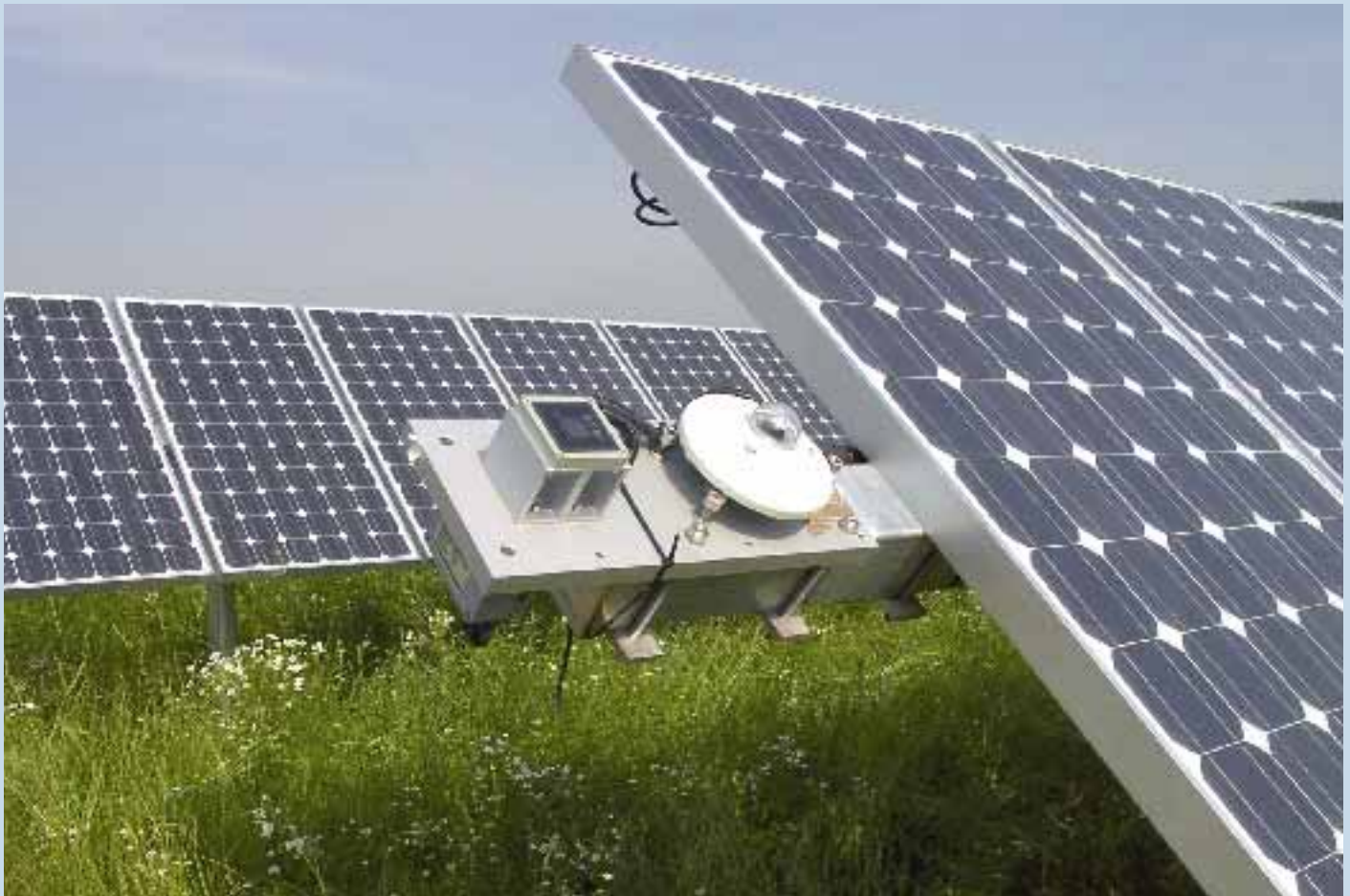
Fig. 1 – Data acquisition systems at a large one-axis tracking PV installation Germany (photo: Fraunhofer ISE).
