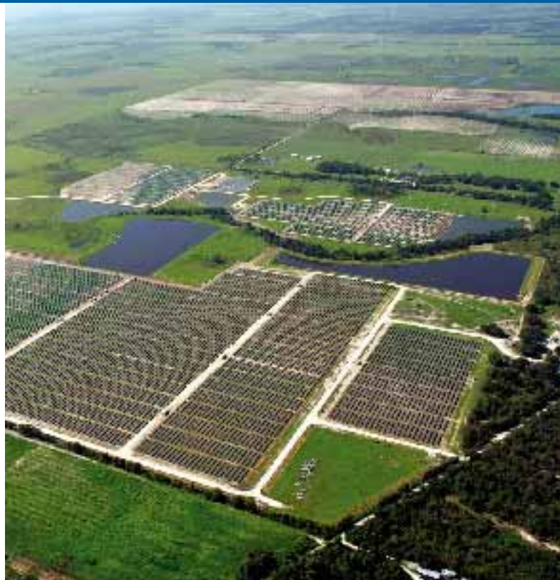
Fig. 1 – DESOTO Next Generation: 25 MW plant in Florida, owned by Florida Power and Light. Annual estimated generation is about 42,000 megawatt-hours or enough power to serve about 3,000 homes. The plant consists of more than 90,500 solar panels.
