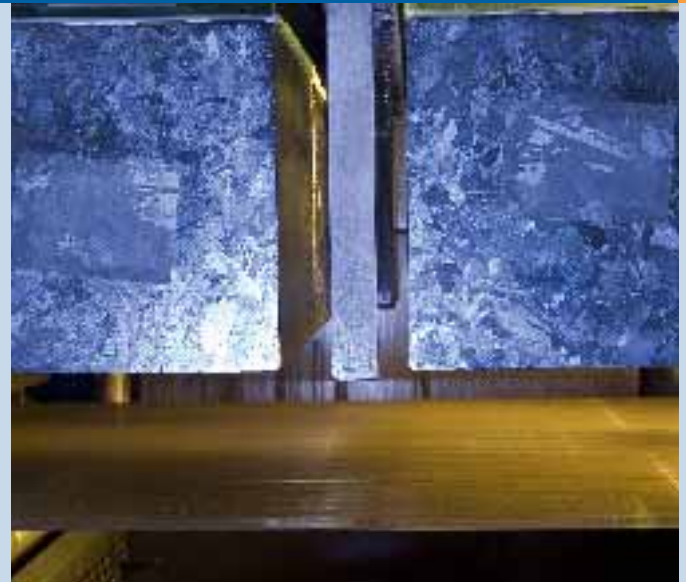
Fig. 5 - Multocrystalline blocks inside a wire saw, PV Crystalox Solar Plc.
