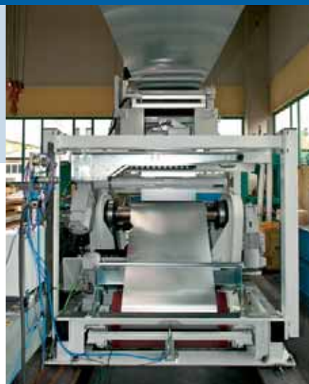
Fig. 2 - Web handling of a Roll-to-Roll tool for thermal treatment of thin film on flexible substrate (Photo: Ebner Industrieofenbau Ges.m.b.H.).
