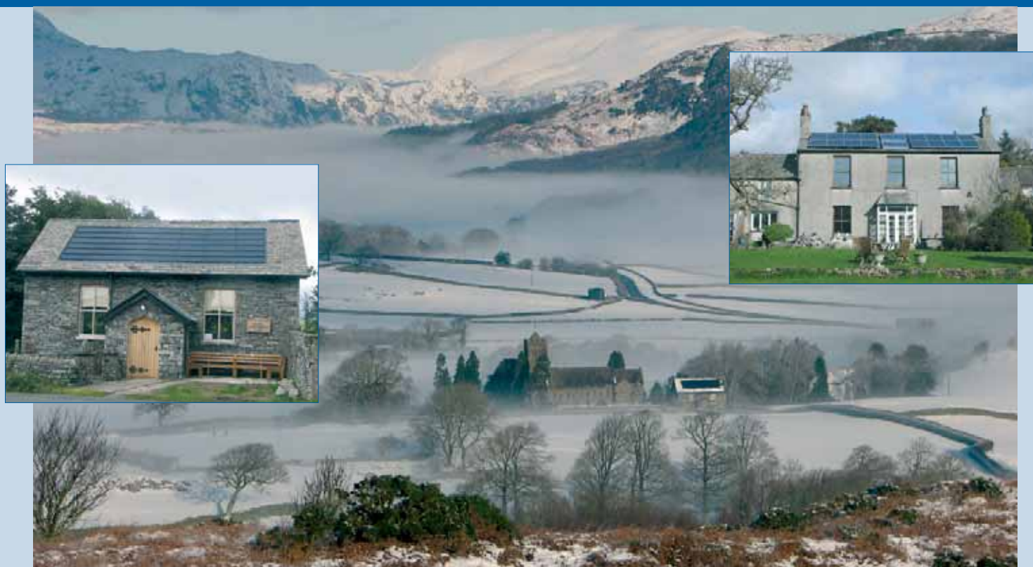
Fig. 1 - PV systems in South Cumbria, UK. The main photo shows PV in the Crake Valley on Lowick Community Hall, next to the church. The Hall, close up on left, has a 3.5 kWp solar PV array integrated into the traditional slate roof. The PV array was installed as part of major refurbishment works to the hall, including a number of other sustainable features. The right hand photo shows a nearby house with a 2.8 kWp PV system and a solar water heating system. (Photos: Donna Munro).
