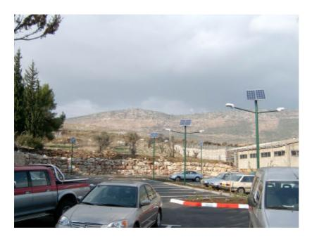
Figure 2: City of Carmiel, in the Galilee. The owners of a supermarket chose PV as the choice for adding lighting to their parking lot, primarily as the least expensive method. The system consists of three double and two single poles, which automatically turn on at sunset and turn off at midnight. [Provided by Solarpower Co.]
