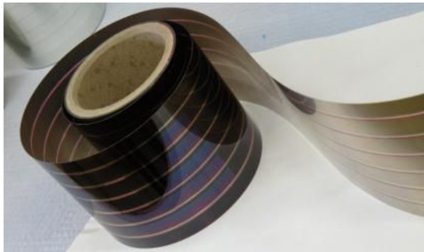
Figure 3: Reel-to-reel printed OPV device fabricated at CSIRO
