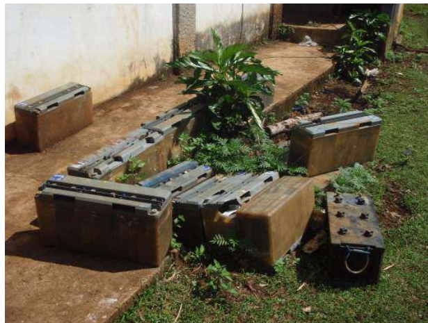
Figure 2. Collected and abandoned batteries for SHS in small, outer island in the Kingdom of Tonga.
