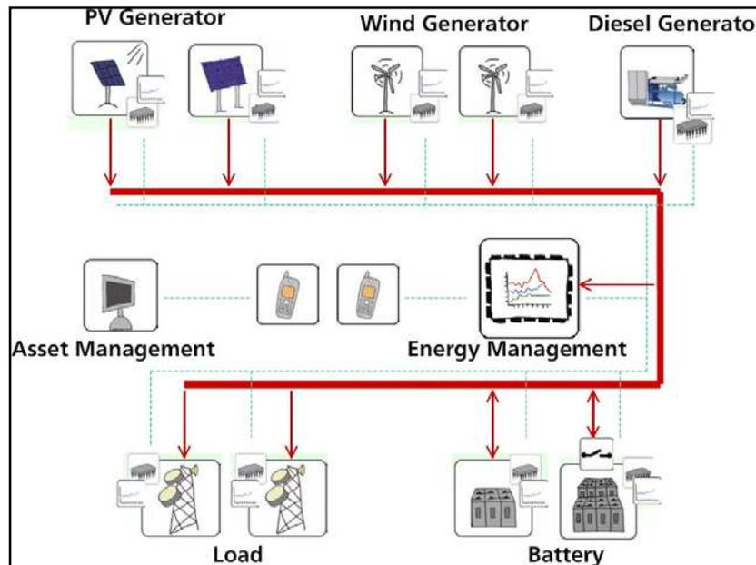
**Figure 16: Extended UESP System with additional generators to supply increased energy demand**
