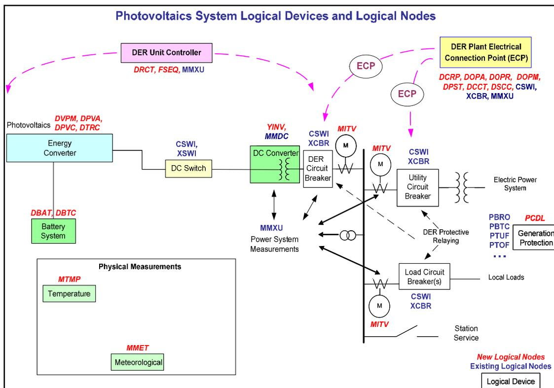
The IEC 61 850 group of standards represents a modern and extendable set of standards for data communication within mini-grids and between mini-grids and the central electric power system that generally conforms to the recommendations of IEEE 1547.3. However there are some implementation issues that affect adoption in PV hybrid mini-grids.
