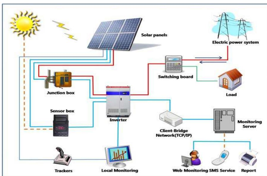
**Figure 8: Typical Layout of a Photovoltaic System in Korea.**
