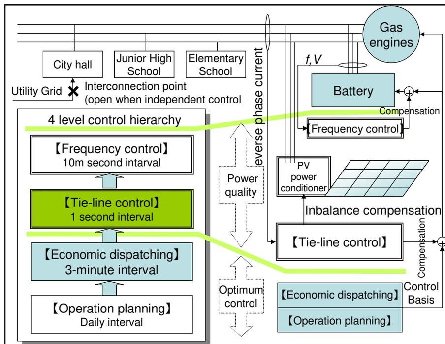
Figure 5: Structure of Hachinohe project control system
