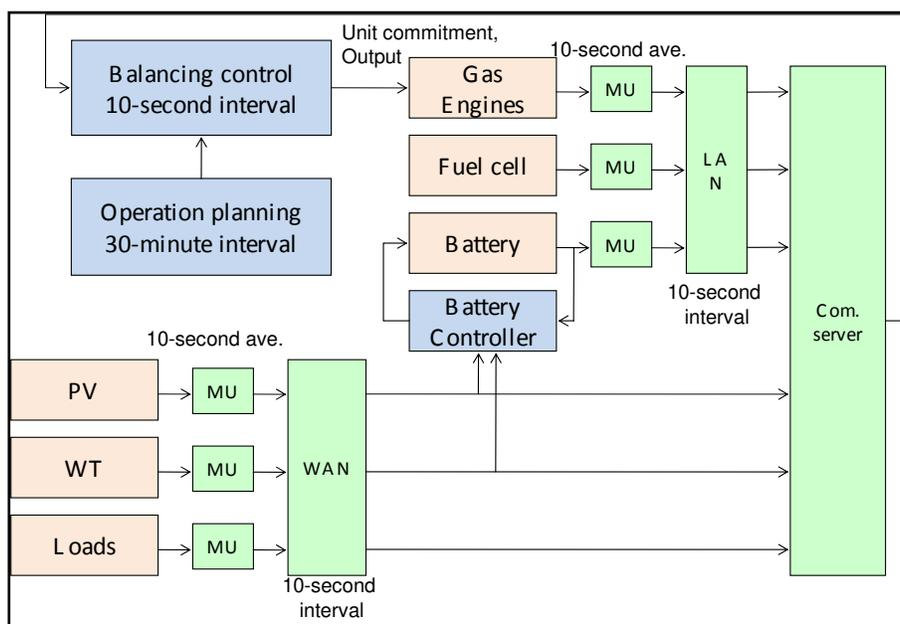
**Figure 6: Structure of Kyotango project control system**
