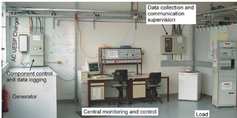
**Figure 20: Picture of the UESP certification laboratory**
