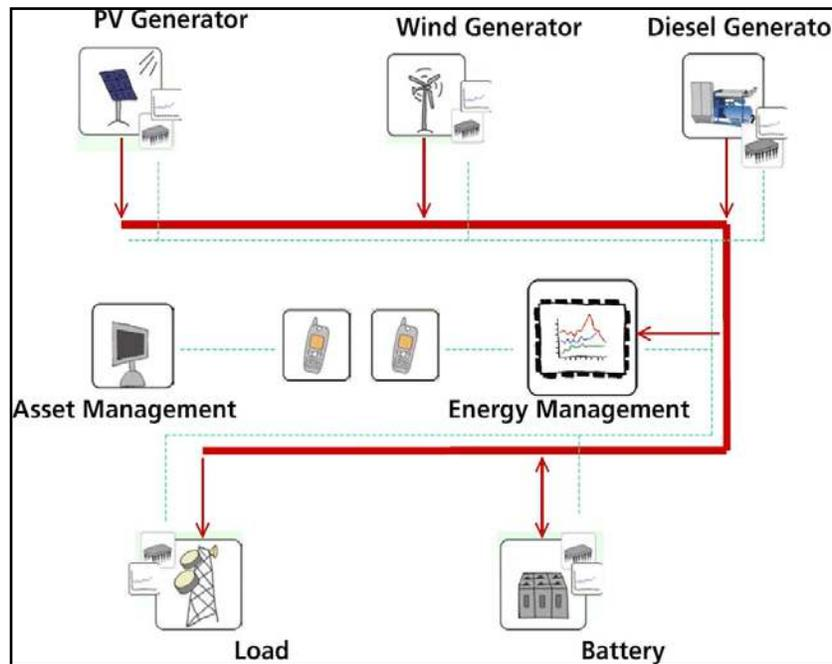
**Figure 15: Simple UESP System for initial supply for telecom load**
