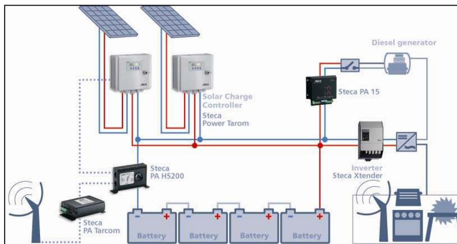
**Figure 1 - Typical Layout of a PV-Hybrid system**
