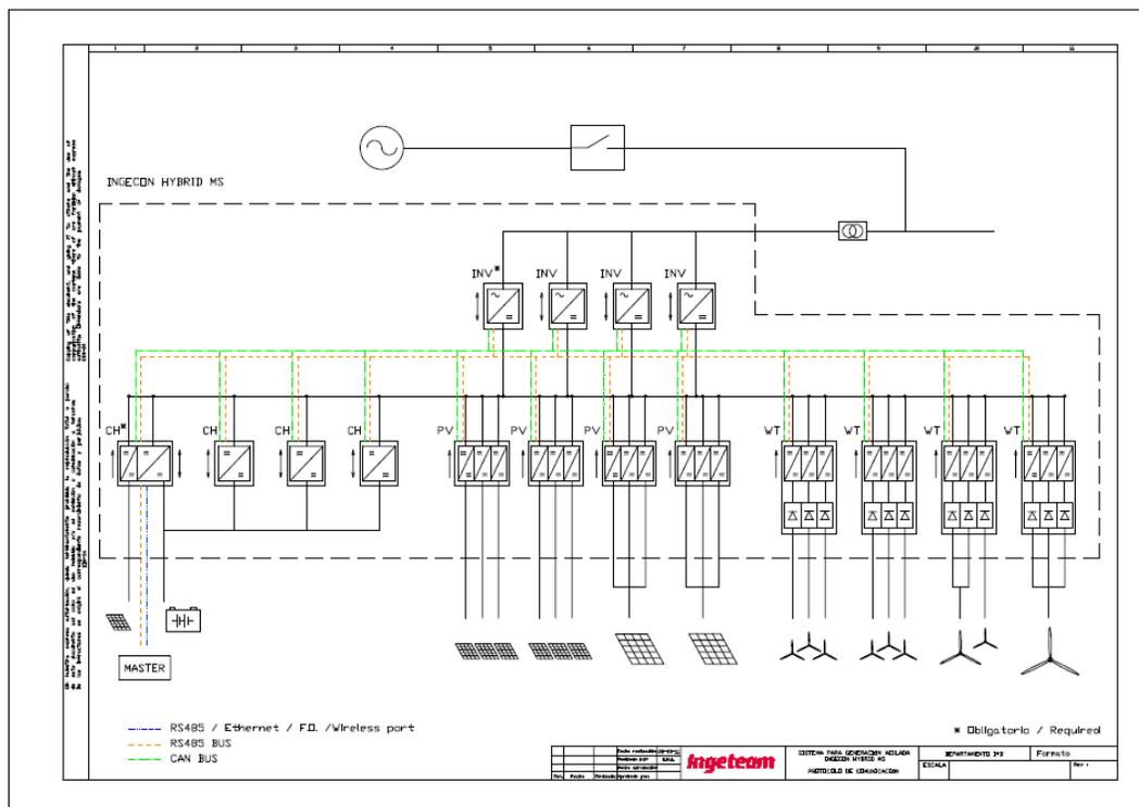
**Figure 14: General layout of an Ingecon system**
