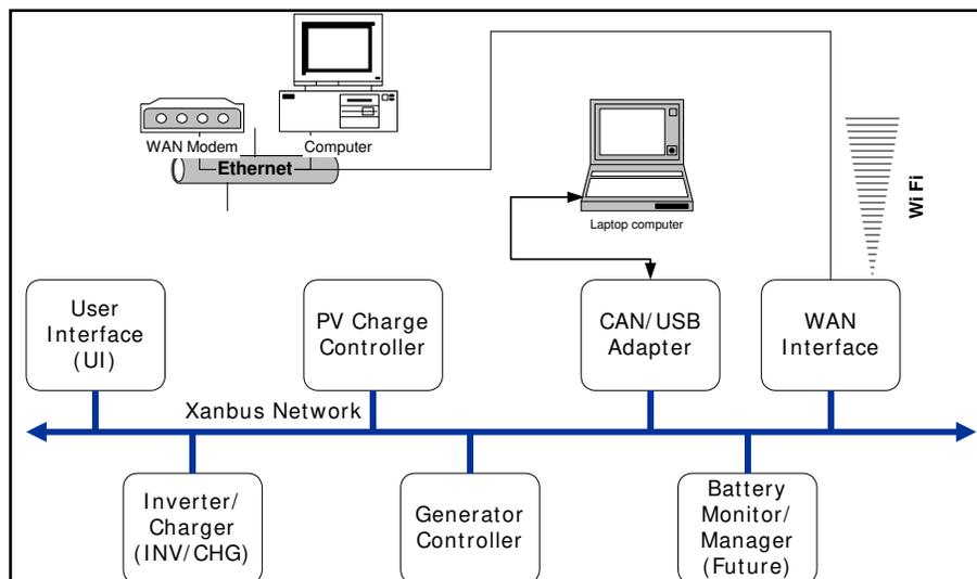
**Figure 9: Functionality of the Xanbus network**
