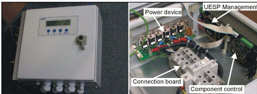
**Figure 18: Example of Steca PowerTarom in UESP Version.**
