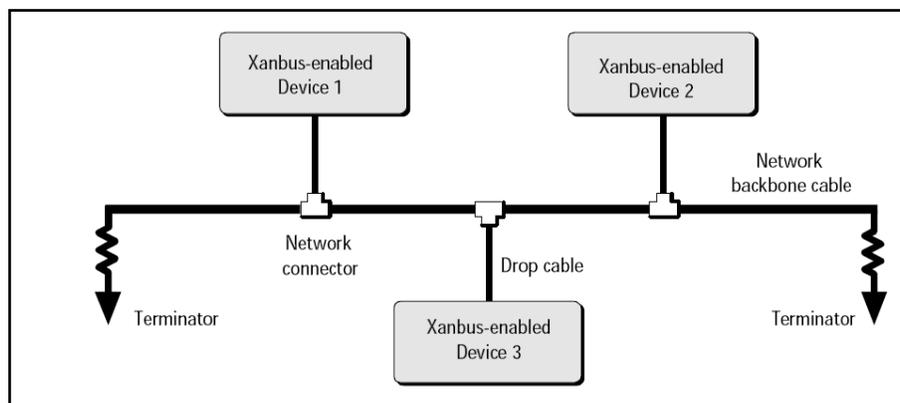
**Figure 10: Multi-drop backbone topology**
