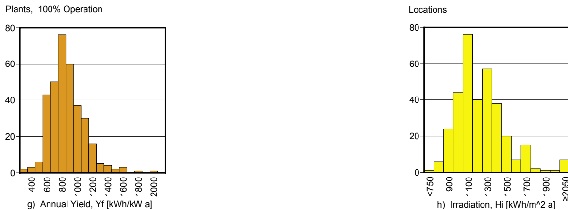
Figures 5.1 and 5.2, Histograms of the mean annual yield and the annual irradiation of all the grid-connected PV plants and locations, adjusted to O = 0 , 100% operation.
