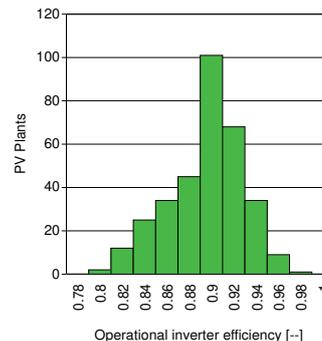
Figure 28, Annual operational inverter efficiency.
