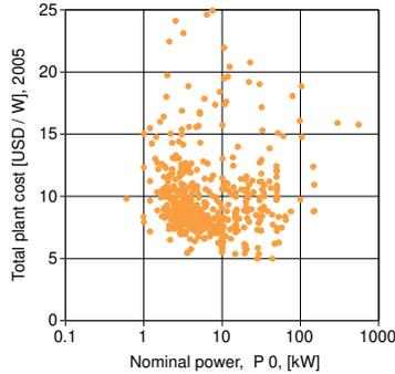
Figure 9, Plant cost to nominal power, logarithmic scale.
