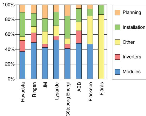
Figure 47, Breakdown of the system cost in percent for 8 Swedish PV systems.
