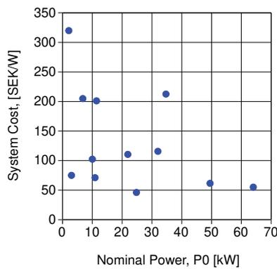
Figure 46, System cost to the installed power for the 12 Swedish PV systems
