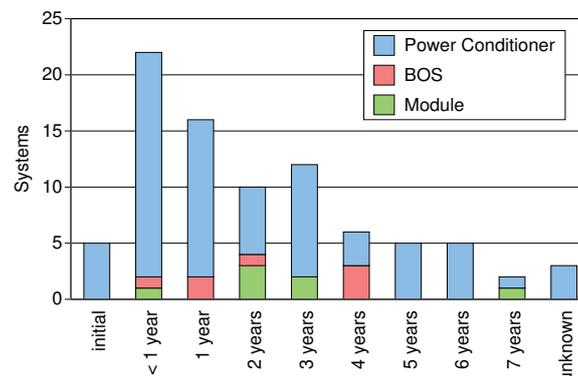
Figure III, Distribution of the operational year of first failure after installation from a survey of 725 small domestic PV systems in Japan.
