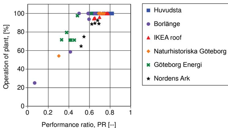
Figure 50, Comparison of the performance to the operation of the plant, six PV plants in Sweden.
