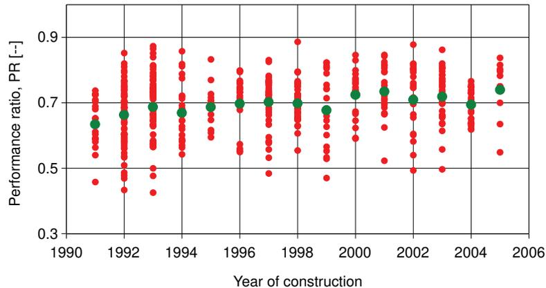
Figure II, Performance ratio over time of the 461 grid-connected PV systems built between 1991 and 2005. Showing the values for each system as well as the annual mean value.
