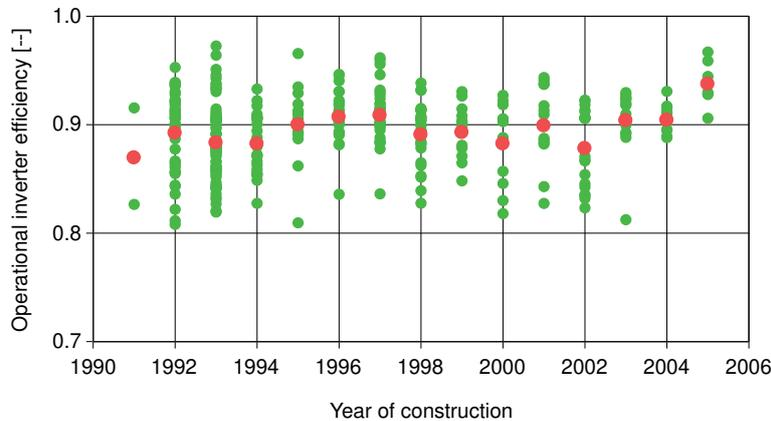
Figure 27, Annual operational inverter efficiency over time.
