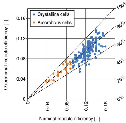
Figure 26, Nominal efficiency to the operational efficiency.
