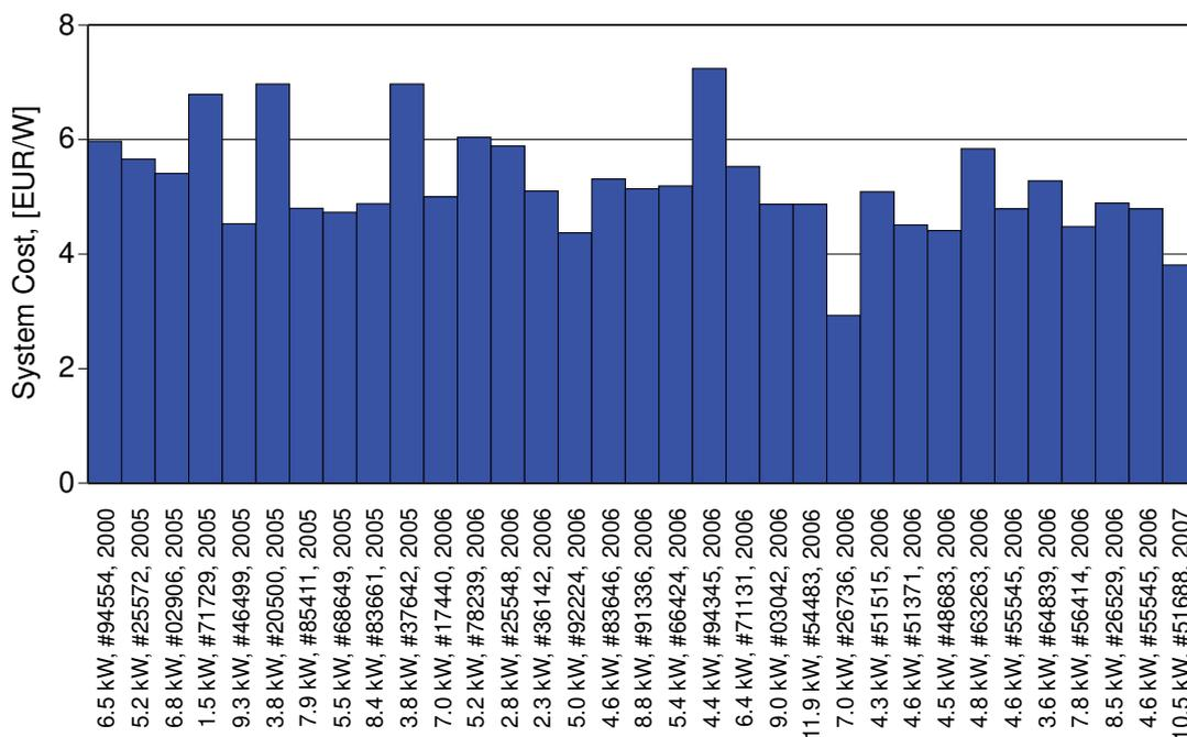
Figure 39, Specific plant cost of 33 grid-connected German residential PV systems, sorted by year of construction.
