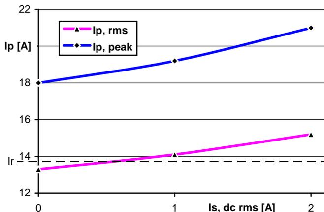
Figure 8 Primary current versus secondary dc component; constant ac load of 12 A
