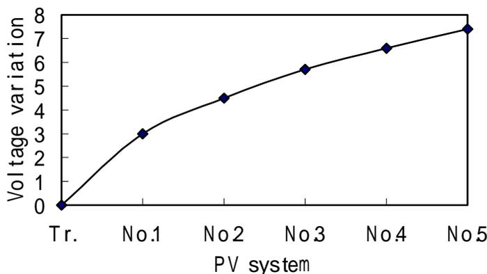
An experimental result of voltage rise at customer's terminals
