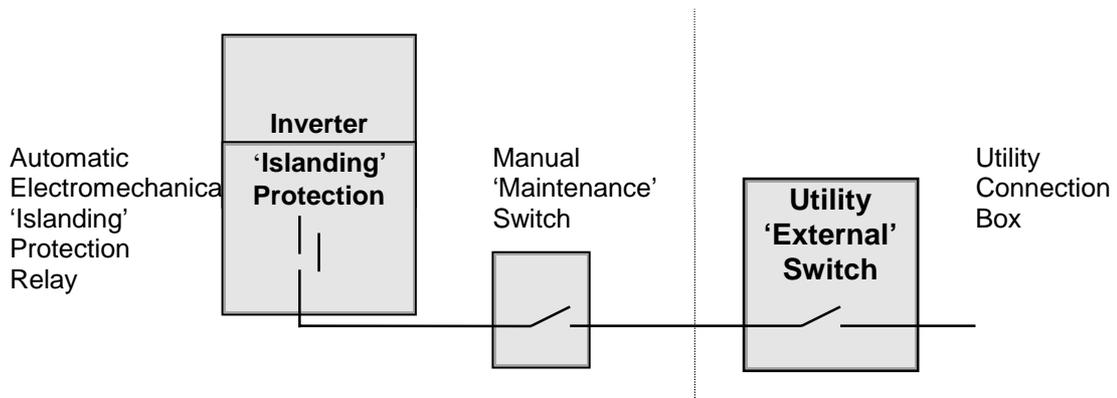
Figure 11.1 External Disconnect Methods
