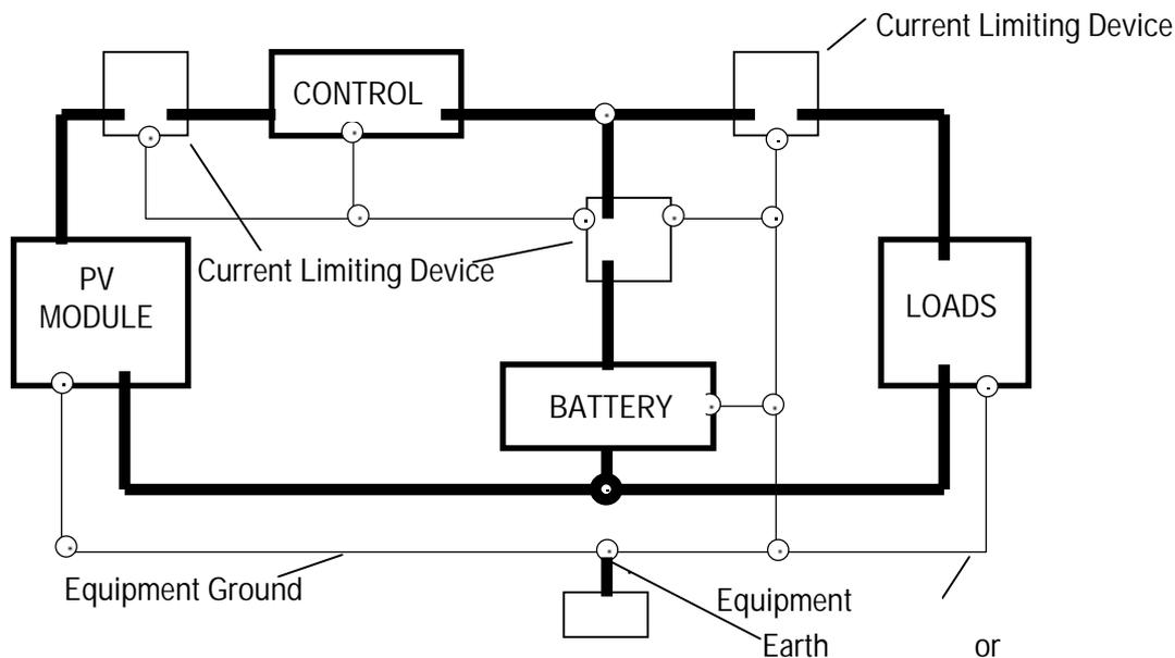
Figure 2. PV System with Equipment Grounding Only
