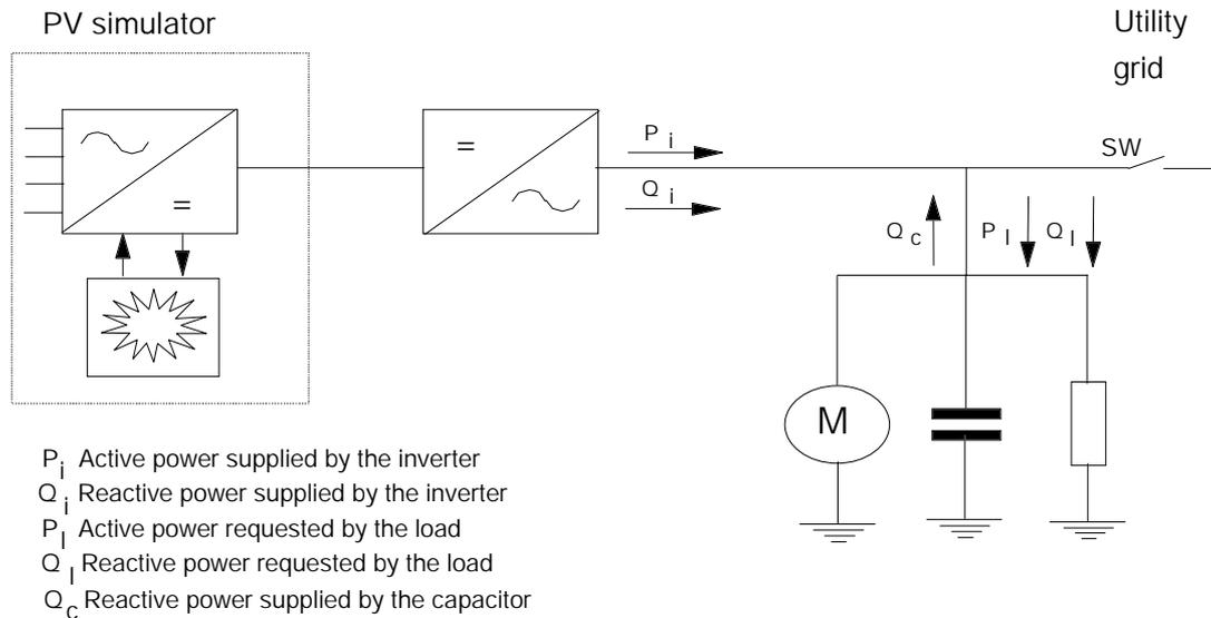
Fig. 2 ENEL test circuit
