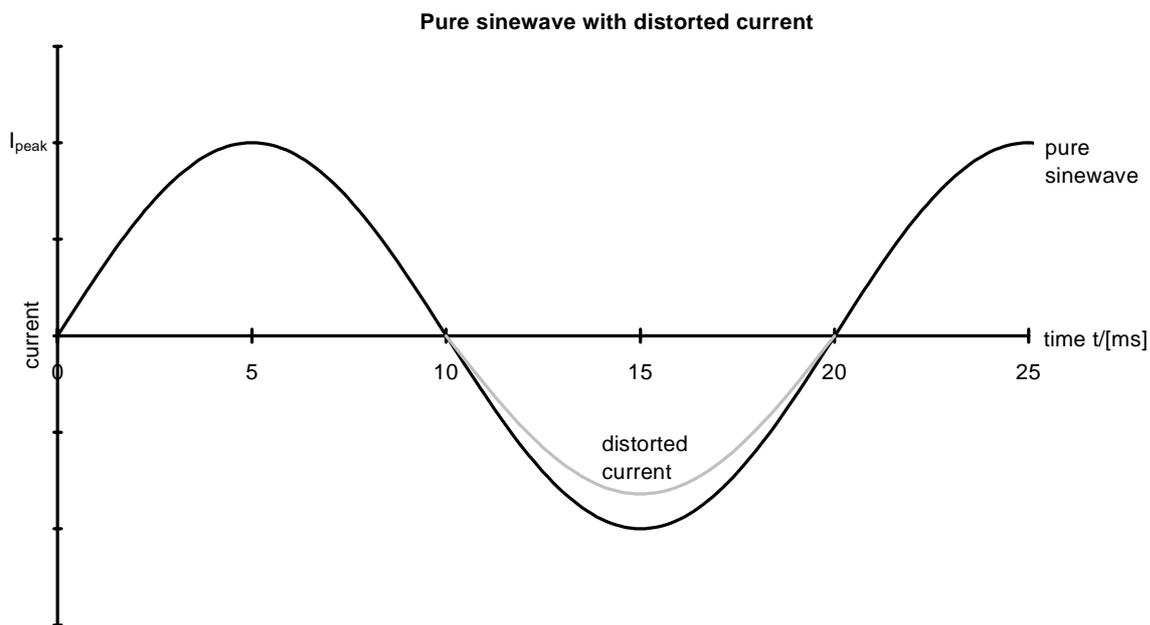
Figure 1 Current with an asymmetrical wave shape.
