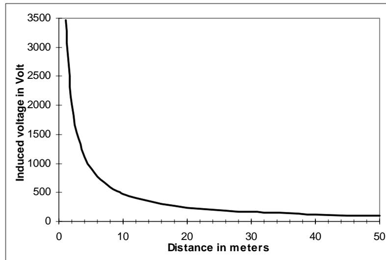
Figure 5 Induced voltage in a loop of 1 m<sup>2</sup> versus the distance between the loop and the lightning current
