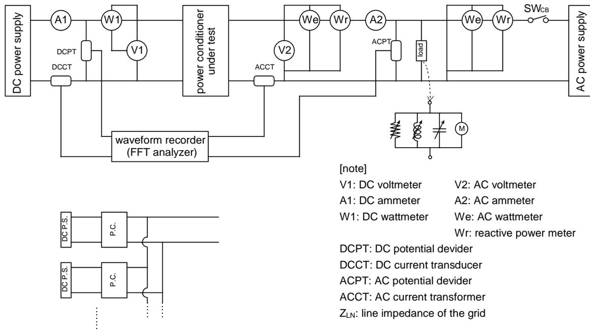
Figure 1 Test circuit for utility connected power conditioners
