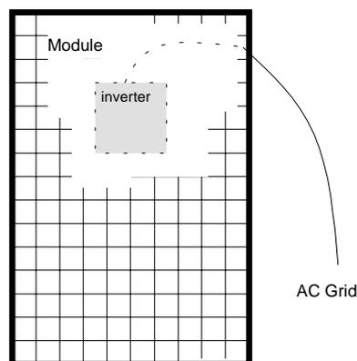
Figure 1 Schematic diagram of an AC Module
