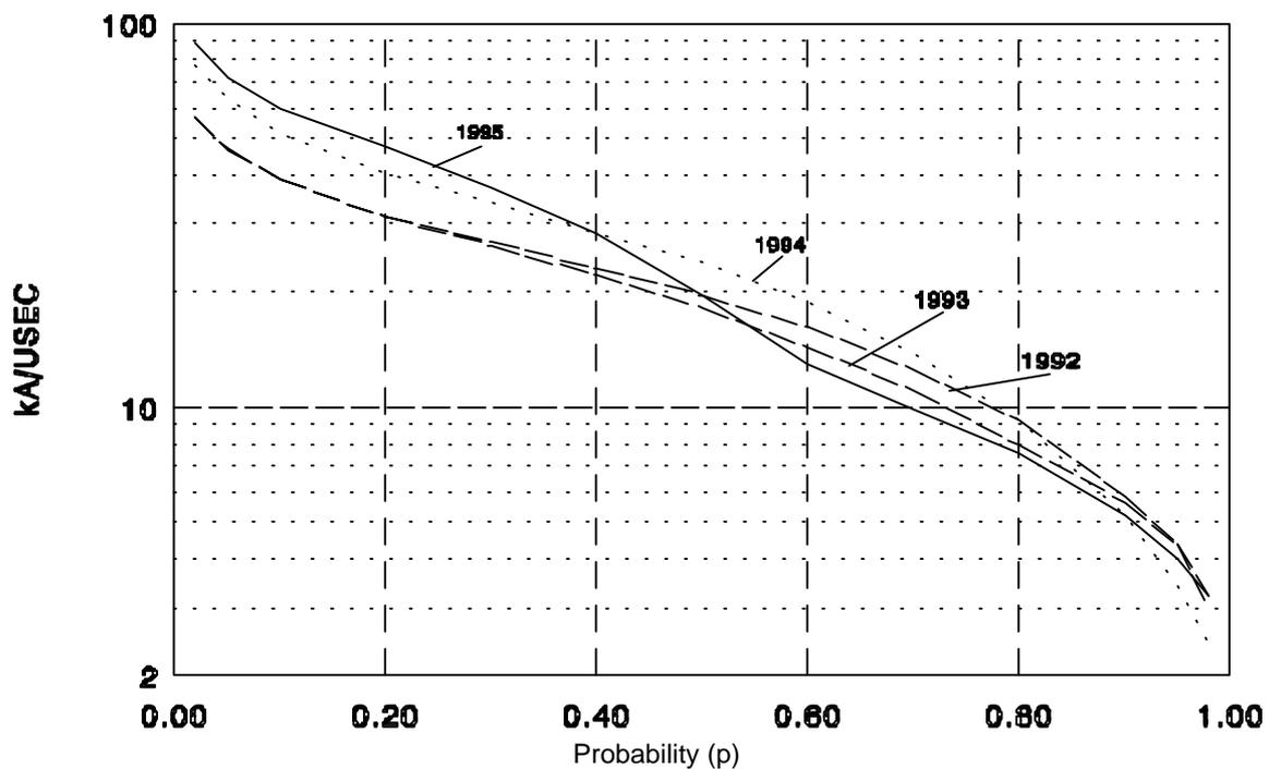
Figure 4 Probability of the di/dt of lightning current
