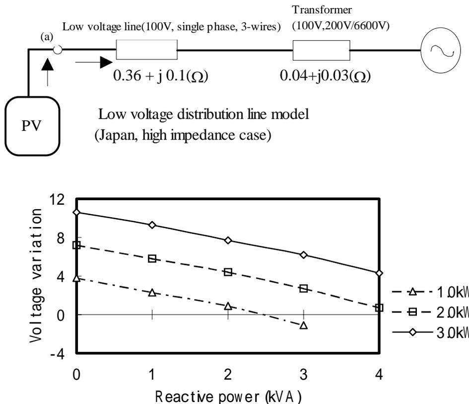
Figure 2 A calculation result on suppression of voltage rise by reactive power control of PV system. Parameter; Real power of PV system
