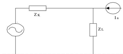
Figure 1 Illustration to calculate the harmonic voltage distortion
