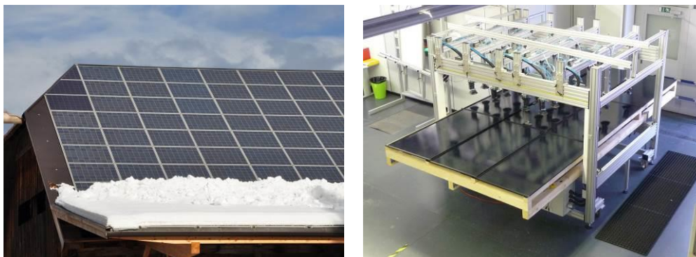
Figure 1: (Left) Non-uniform snow load on PV roofing slates and (right) mechanical load test imposing a uniform load onto a PV panel. (Source: SUPSI)
