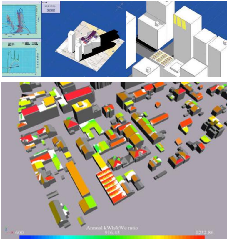
Figure 5: Simulated irradiance on the building envelope for prediction of generated power [ https://www.lapsys.co.jp/english/products/pro.html ] (top) and simulated annual solar energy on rooftops of a neighbourhood [ https://www.cstb.fr ] (bottom).
