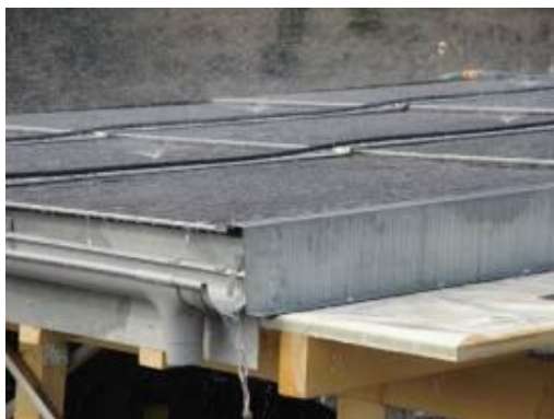
Figure 2: Wind-driven rain test at SUPSI. (Source: SUPSI)
