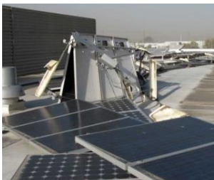
Fig. 10: Destroyed system after high wind load [18].
