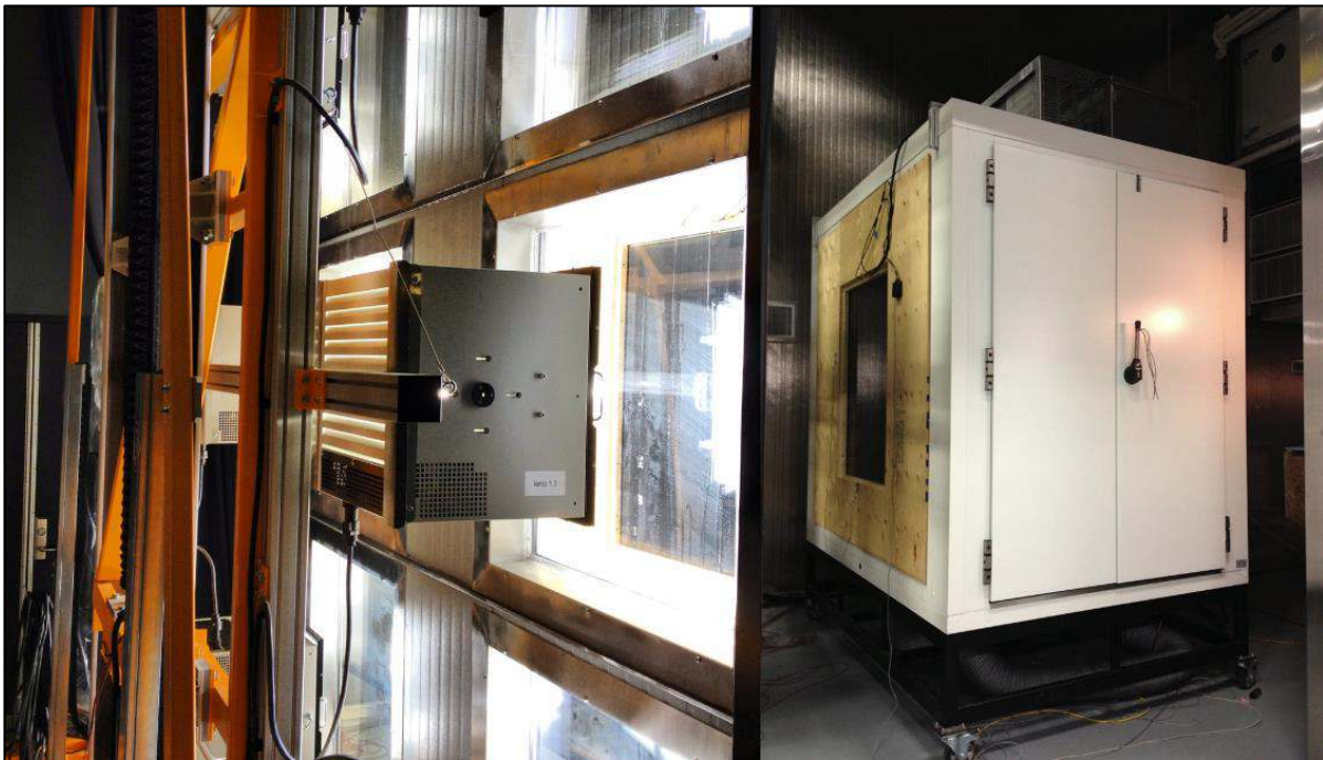
BIPV window Solar Heat Gain Coefficient (SHGC) characterization at Concordia University's Solar Simulator and Environmental Chamber laboratory (Source: K.Kapsis, 2019).
