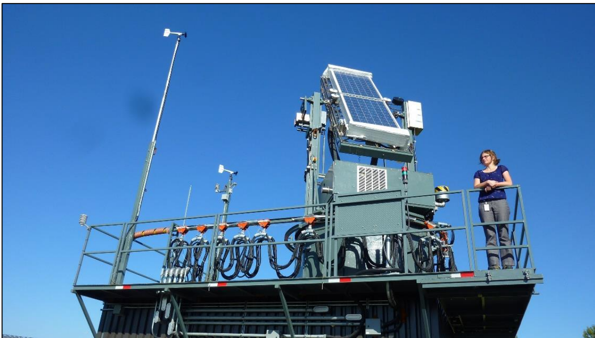
Outdoor BIPV annual electricity yield testing at Natural Resources Canada’s CanmetENERGY research centre in Varennes (Source: Natural Resources Canada, 2019).
