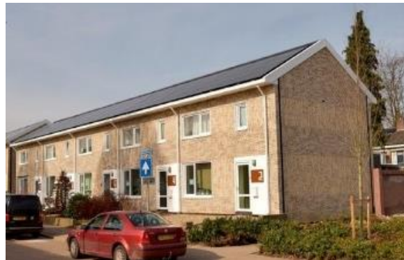
Figure 8: Example of a BIPV roof for terraced houses (new build)
