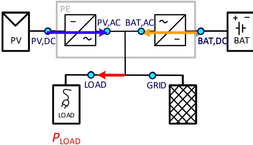
$$P_{BAT2AC}(t) = \frac{P_{BAT,AC}(t)}{\eta_{BAT2AC} \left( \frac{P_{BAT,AC}(t)}{\eta_{AC2BAT}(P_{BAT,AC}(t))} \right)}$$
