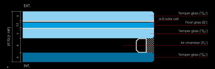
Picture on the left shows a typical amorphous Silicon double glazing configuration, as a reference.
