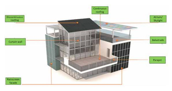
Fig. 1 - Illustration of BIPV installation scenarios categorized in activity B.2. (Source: SUPSI).
