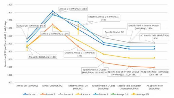
Fig. 3 - Detailed analysis of the contribution of each yield assessment modelling step from GHI to Alternating Current (AC) specific yield for the Bolzano site. The orange dots represent measured values over 2011-2019 with σ.
