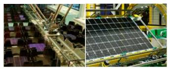
Fig. 6 - EGP 3SUN PV module factory: HJT bifacial cells' and modules' assembly lines (Photos: EGP).
