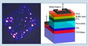
Fig. 5 - (Left) Lock-in thermography image of a semi-transparent perovskite solar cell exposed to a reverse bias of -3V showing hot-spot/shunt formation over the entire cell area. (Right) Schematic of a semi-transparent perovskite solar cell architecture, such as it would be used in a tandem cell configuration (with the Si bottom cell replacing ITO/Glass) (Source: EPFL/CSEM).
