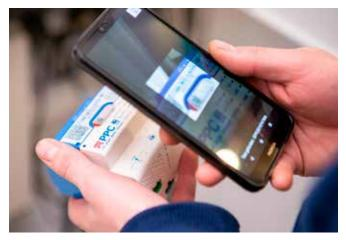
Fig. 3 - Registration process for a Smart Meter Gateway before installation: A PIN/TAN registration process for the installation of the Smart Meter Gateways implemented in Germany to improve the security of the smart grid information system (Photo: © PPC AG).
