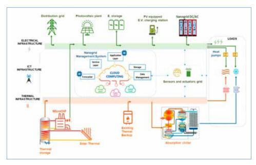
Fig. 3 - ENEA experimental multivector smart nanogrid layout.
