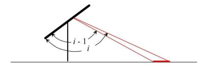
Figure 48: Field-of-view of the ground for a one-degree segment depicted by the angles *i* and *i*-1.
