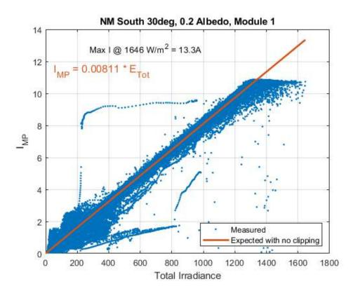
Figure 29: Example scatter plot of 1-min  $I_{mpp}$  values from a bifacial module in New Mexico plotted against total irradiance (front + rear). Red regression line extends to the maximum measured total irradiance. Maximum 1-min current is estimated from the  $I_{mpp}$  value at the maximum total irradiance.
