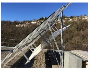
Figure 84: Bifacial test stand installed at SUPSI within the Swiss Project ENHANCE. (top row) Configuration including 3 monitored bifacial modules, 2 dummy modules, and 1 reference monofacial module in open-rack layout. (bottom row) Front view and side view, respectively, of white reflectors mounted behind bifacial PV modules.
