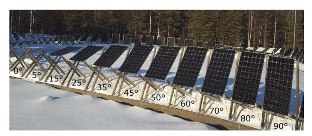
Figure 97: Photograph of the selected section of Solvåg with the inclination presented below each module.
