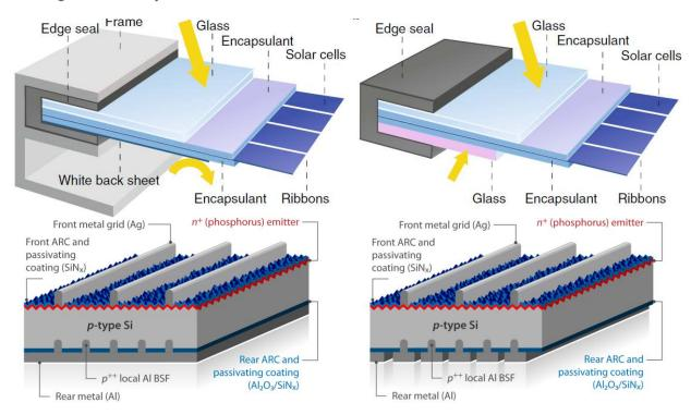
Figure 11: Differences between PV modules: monofacial (upper left) and bifacial (upper right) and differences between solar cells: monofacial PERC (lower left) and bifacial PERC+ (lower right).
