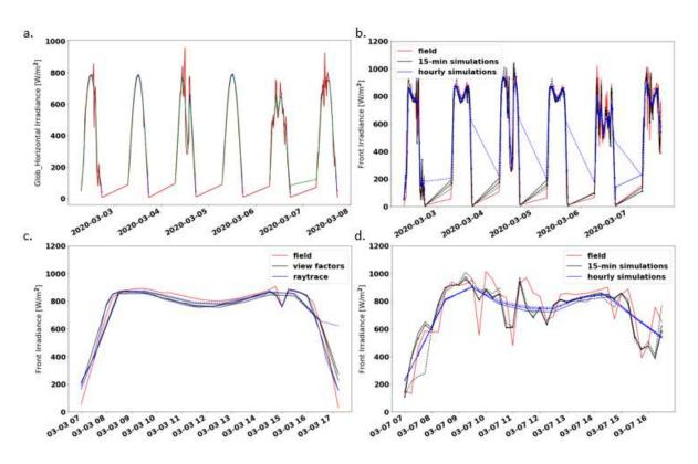
Figure 63: Results for optional simulation 2, including four view factor and 2 raytracing modeling tools. (a) Global Horizontal data was used to properly align the results of all the tools. (b) Front irradiance results for the week modeled. (c) Close-up on simulations and field data for one sunny day and for (d) one variable-cloudy day.
