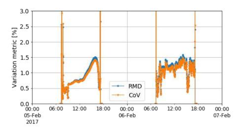
Figure 24: Spatial variation in total irradiance measured at Sandia during two days in New Mexico USA.
