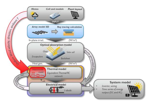
Figure 56: Structure of the Imec Energy Yield Modeling framework.
