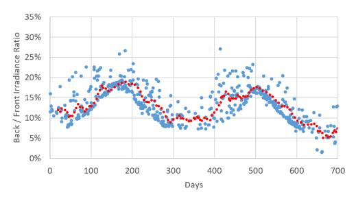
Figure 72: Rear-side to front-side irradiance ratio over the first two years of operation. Blue dots denote daily values, red dots form a 20-day moving average.
