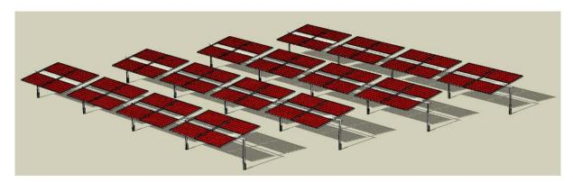
Figure 57: Example of PV array 3D model used for bifacial energy yield simulations within the Imec Energy Yield Modeling framework.
