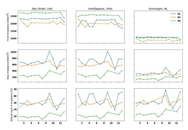
Figure 60: Cumulative yearly results for front Irradiance, rear irradiance, and bifacial gain (rear / front irradiances) for the three cities with different climates. Simulation 1 (blue) is fixed tilt Equator facing, Simulation 2 (orange) is fixed tilt West facing, and Simulation 4 (green) is single-axis tracking. The results are shown on the x-axis in the same order between plots, but they are in random order relative to the way they are presented in the report to anonymize them.
