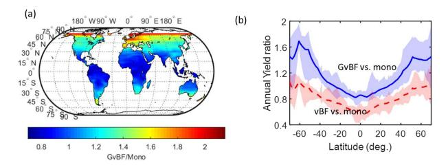
Figure 41: (left) Worldwide annual yield ratio between Gv-BF and monofacial solar cell. (right) For various latitudes, ratio of annual yields of GvBF (R=0.5) vs. monofacial plant, and of v-BF (R=0.3) vs. monofacial plant are shown by solid and dashed lines, respectively. The monofacial system includes a 10% soiling loss. The shaded regions, along with the lines, represent the spread in data for various longitudes.
