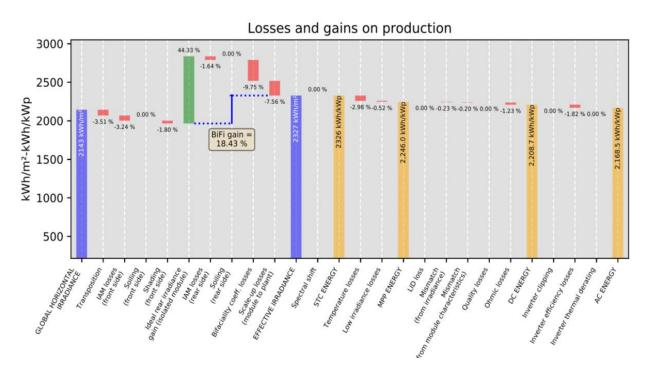
Figure 51: Losses and gains on production calculated by PVNOV.
