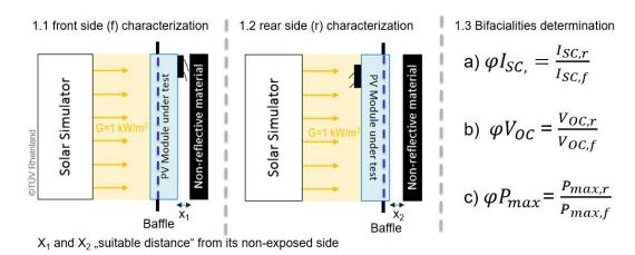
Figure 13: IEC TS 60904-1-2 test method for IV measurement of bifacial PV modules: Determination of bifaciality factor at STC. An opaque non-reflective background ensures less than 3 W/m<sup>2</sup> at any point on the non-illuminated side of the PV device.
