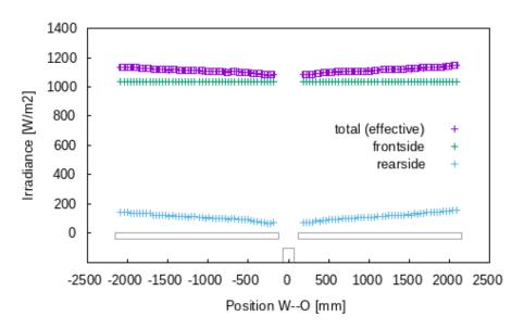
Figure 25: Irradiance levels across two modules on a horizontal single-axis tracker (2P) for one exemplary time step (noon at June 21<sup>st</sup>). Rear-side irradiance shows a mostly linear decrease from the edge towards the center of the tracker table.
