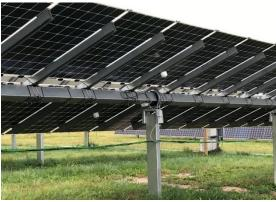
Figure 103: (left) Direct normal, diffuse horizontal, and global horizontal radiation measured at the campus solar radiation monitoring station. (right) Spectrally flat class C pyranometers installed on the backside of a fixed tilt array T11.
