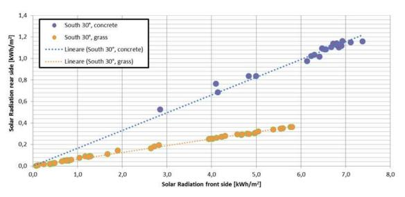
Figure 108: Trend of daily incident solar radiation on front and rear side with change in ground albedo under the PV system.
