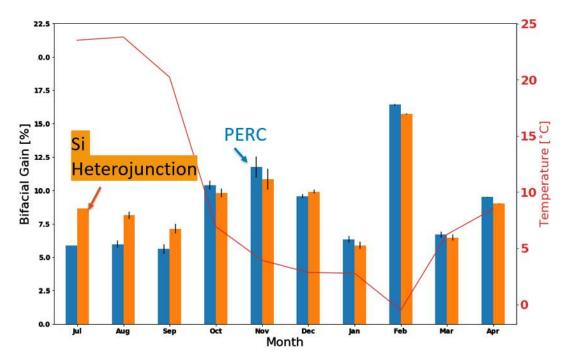
Figure 93: Monthly bifacial gain for two of the PERC technologies and a Silicon Heterojunction technology for six months of collected data. The alternating effects of temperature and snow are visible before and after beginning of October.
