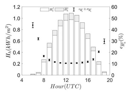
Figure 86: Available solar irradiation at module 16-113-A1 on day number 227. Left y axis: Columns chart stacking of the hourly front solar irradiation  $H_h^f$  and mean rear solar irradiation  $\overline{H_h^r}$ . Right y axis: Fraction of mean rear irradiation  $\epsilon_{\overline{H_h^r}}$  and standard deviation  $\sigma_{\overline{H_h^r}}$ .
