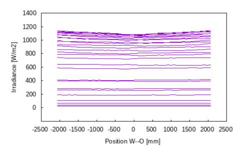
Figure 26: Irradiance levels across two modules on a horizontal single-axis tracker (2P) for all time steps of one day (June 21<sup>st</sup>). Non-uniformity is more pronounced at high irradiance levels (i.e., around noon) when the tracker position is close to horizontal.
