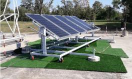
Figure 107: Bifacial PV system under test; South-facing PV module on light grey concrete tilted 30°(left); South-facing PV modules on synthetic green grass tilted 30° (right).
