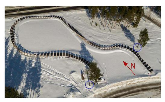
Figure 95: Birds-eye view of the Solvåg solar site in March 2018. The red arrow denotes the North direction, and the blue circles mark trees that have been cut (September 2018) to limit issues with direct shadowing. Photo: Mikael Sundqvist (P-town Productions).
