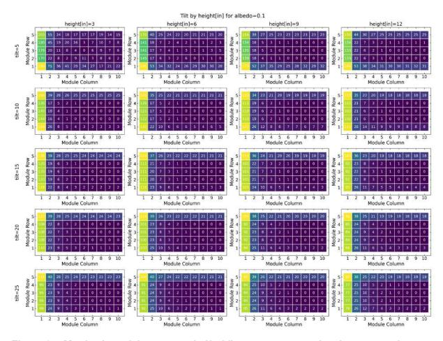
Figure 34: Matrix view of the western half of five-row systems showing percent increase in rear-side irradiation as compared with the center-most module. Each run is at a different tilt angle and pitch (row in the matrix) and module height (column in the matrix).
