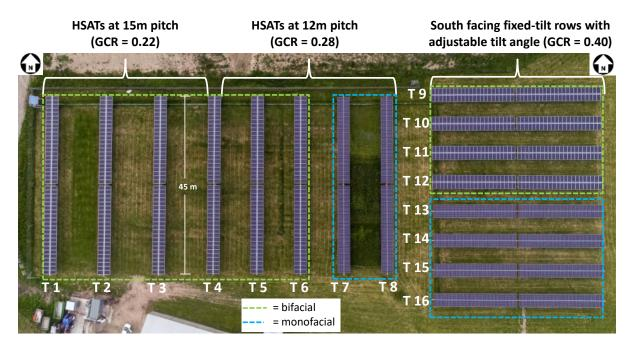
Figure 100: Aerial view of the bifacial test facility at DTU. Annotations show tracker number, substructure type, pitch, and module type.
