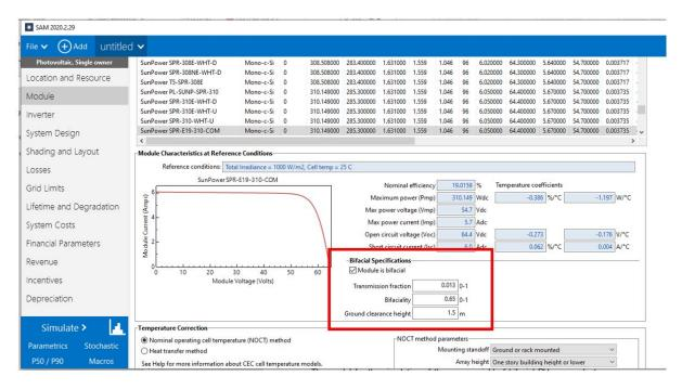
Figure 52: System Advisor Model bifacial functionality for module and simulations.
