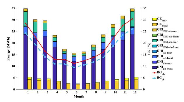
Figure 54: Breakdown of absorbed irradiation, amount of generated electricity (GE) and bifacial gain related to absorbed irradiation (BG<sub>ab</sub>) and bifacial gain related to generated electricity (BG<sub>el</sub>) for the location San Felipe, Chile.
