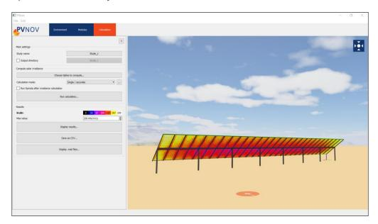
Figure 50: Calculation of irradiance for each module in a row using PVNOV.
