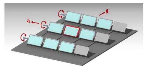
Figure 82: Measurement set-up with permanently turning modules. The center, which is best suited to represent the actual conditions in real installations, is outlined in red.
