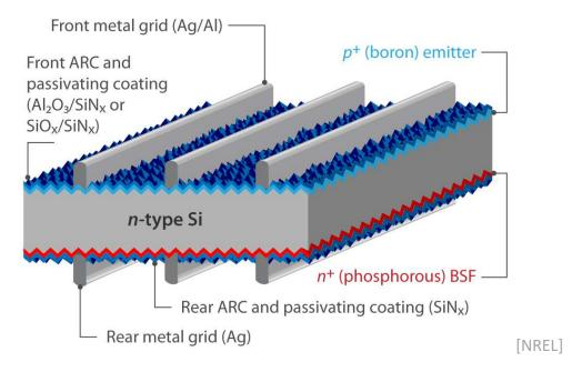
Figure 4: Typical bifacial n-PERT cell scheme.
