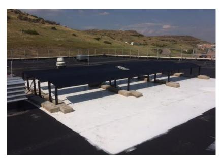
Figure 45: Fixed-tilt testbed for optional simulation 1
