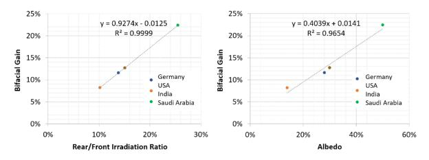
Figure 81: Correlation between rear/front irradiation ratio (left) and albedo (right) and bifacial gain.
