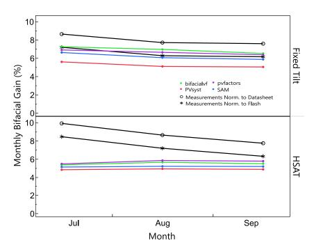
Figure 105: Simulated and measured bifacial gains of two system types (fixed tilt and HSAT) over grass for the three month period shown in Figure 102.
