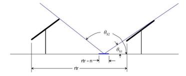
Figure 47: Field-of-view angles for determining the VF for the diffuse sky radiation incident a ground segment.
