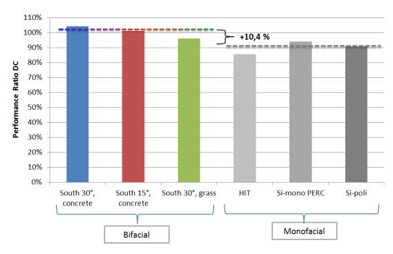
Figure 110: PR<sub>DC</sub> of the bifacial modules in the three test configurations and the highest-performing monofacial modules monitored by RSE.
