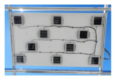
Figure 20: Rear view of the Sandia irradiance distribution module (IDM) showing the placement of the ten reference cells.
