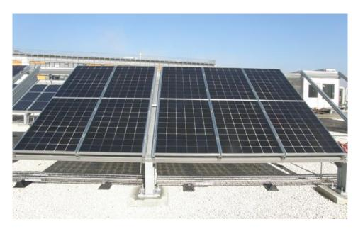
Figure 70: Front view of PV bifacial modules under test at INES site.
