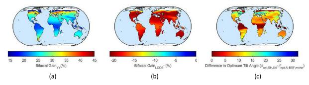
Figure 42: Global maps comparing bifacial gain in (a) yearly energy yield, (b) LCOE\*, and (c) difference in optimum array tilt angle for Al-BSF monofacial ( $\beta_T = 0.41\%/^{\circ}C$ ) vs silicon heterojunction bifacial ( $\beta_T = 0.26\%/^{\circ}C$ ). Note that  $R_A = 0.5$  and  $M_L = 15$ .
