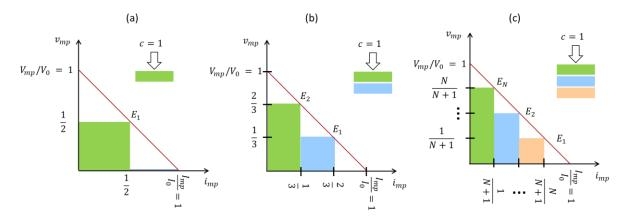
Figure 7: SQ triangle for monofacial cells: (a) Single junction, SJ; (b) double-junction, DJ, and (c) multi-junction PV. For a two-terminal configuration, the bandgaps are optimized to produce equal current.
