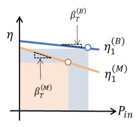
Figure 10: Bifacial gain is defined by the ratio of boxes in the  $\eta-P_{in}$  plane. In intrinsic thermodynamics ( $\beta_T$ =const), temperature-dependence erodes bifacial gain. In practice,  $\beta_T^{(B)} < \beta_T^{(M)}$  further improves bifacial gain.
