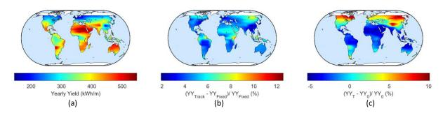
Figure 43: (a) Yearly energy yield for tracking bifacial PV with temperature-dependent efficiency ( $\eta(T)$ ). (b) Percentage change in yearly energy yield of tracking bifacial PV vs. N-S fixed-tilt bifacial PV. (c) Percentage change in YY for tracking bifacial PV with temperature-dependent efficiency and constant efficiency ( $\eta$  STC).
