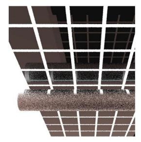
Figure 46: (left) Model in bifacial\_radiance of the NREL bifacial experimental single-axis tracking field array in Golden, Colorado. (right) Close-up on a module modeled cell-by-cell, with round torque-tube and glass.
