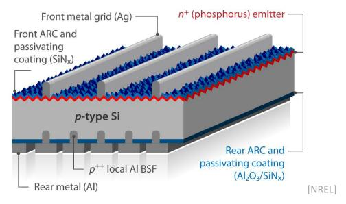
Figure 3: Typical bifacial p-type PERC+ cell scheme.
