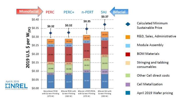
Figure 2: Monofacial versus bifacial module manufacturing cost calculation.
