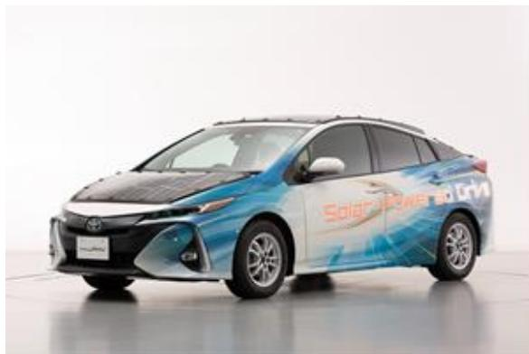
**Fig. A-3 PV-powered Prius-HEV (Toyota)**
