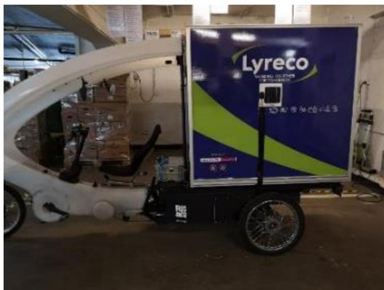
Fig. 3.3-8 The «Rikscha Taxi» with a cargo box showing the left irradiance sensor.
