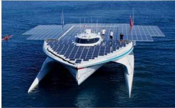
Fig. 1.1-9 A boat proof of concept - Tûranor form PlanetSolar [9]
