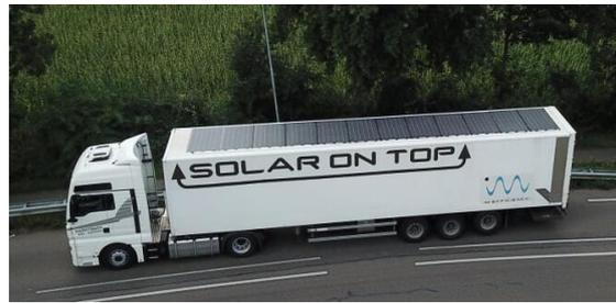
**Fig. B-2 PV truck trailer**
