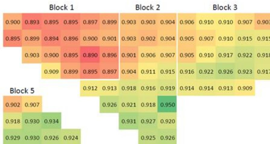
**Figure 17: Data showing uneven power reduction across a large PV plant [51].**
