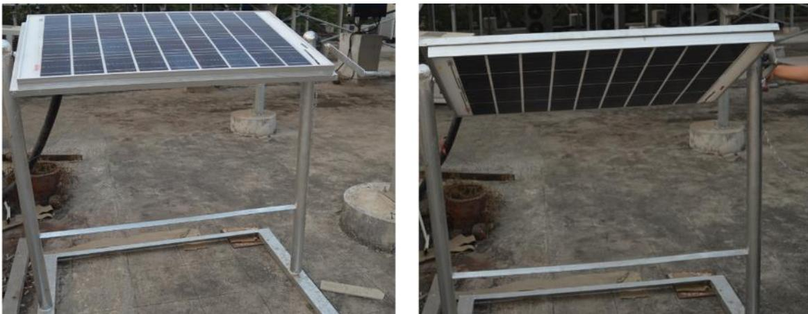
**Figure 36:** The photograph on the left shows the inverted module during the day, and the photograph on the right shows it during the night.
