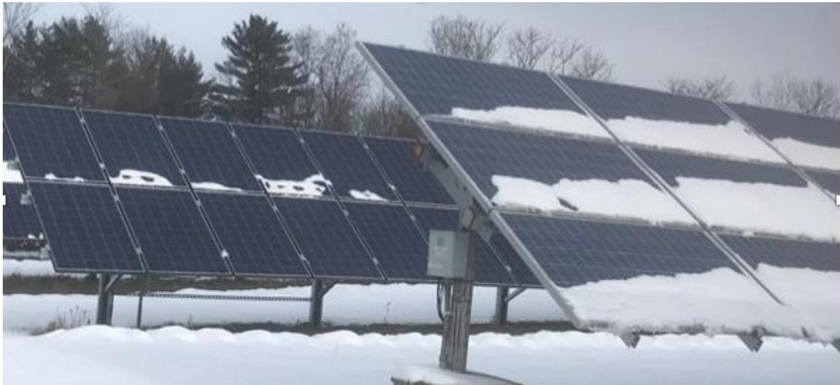
**Figure 56: Two adjacent PV systems set at the same tilt angle but with different module orientations create an ideal experimental set-up for investigating the impact of orientation on snow shedding. As shown above, orientation can impact shedding rates, although more research is needed to investigate temperature-dependency and the role of bypass diodes [160].**
