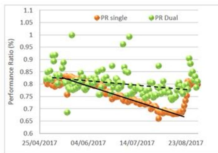
**Figure 41: Daily performance ratio trends for single axis and dual-axis trackers during the 2017 dry season illustrates higher soiling rates on the single axis tracker.**
