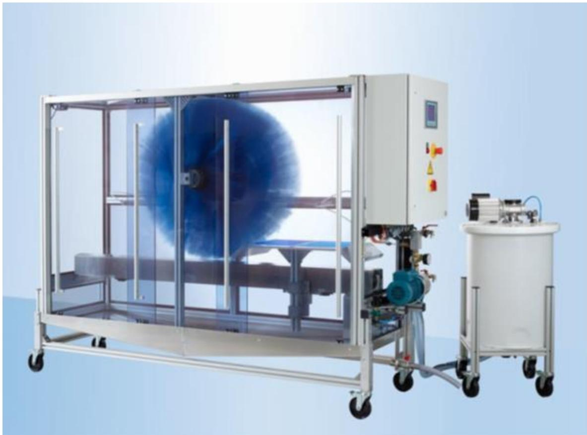
Figure 45: Laboratory car wash for testing the scratch resistance of coatings in accordance to ISO 20566 [149].
