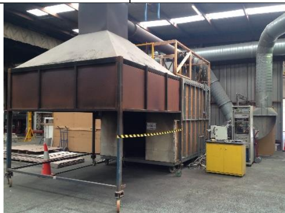
Photo of the ISO 9705 test rig.
