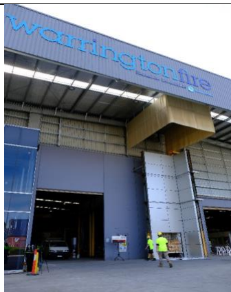
Photo of façade test rig.
