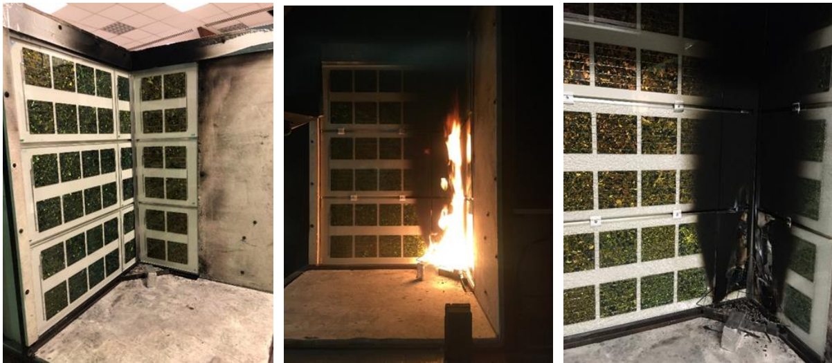
Figure 10 Fire resistance bench test requirements applied to BIPV components (SBI).
