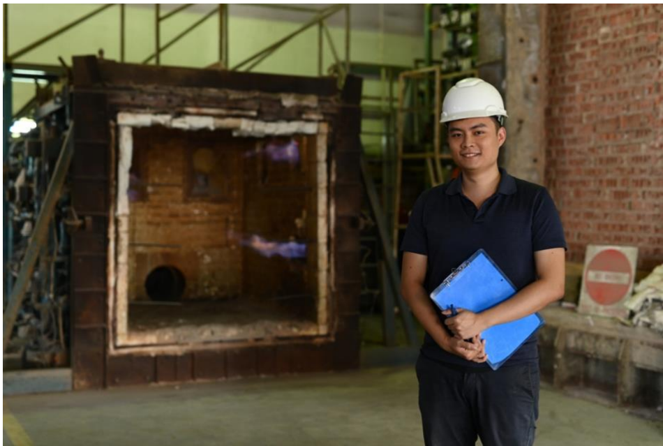
Figure 26: Furnace for fire-resistance testing.
