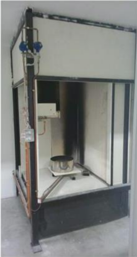
Figure 12: SBI test facility (UNI EN 13823).
