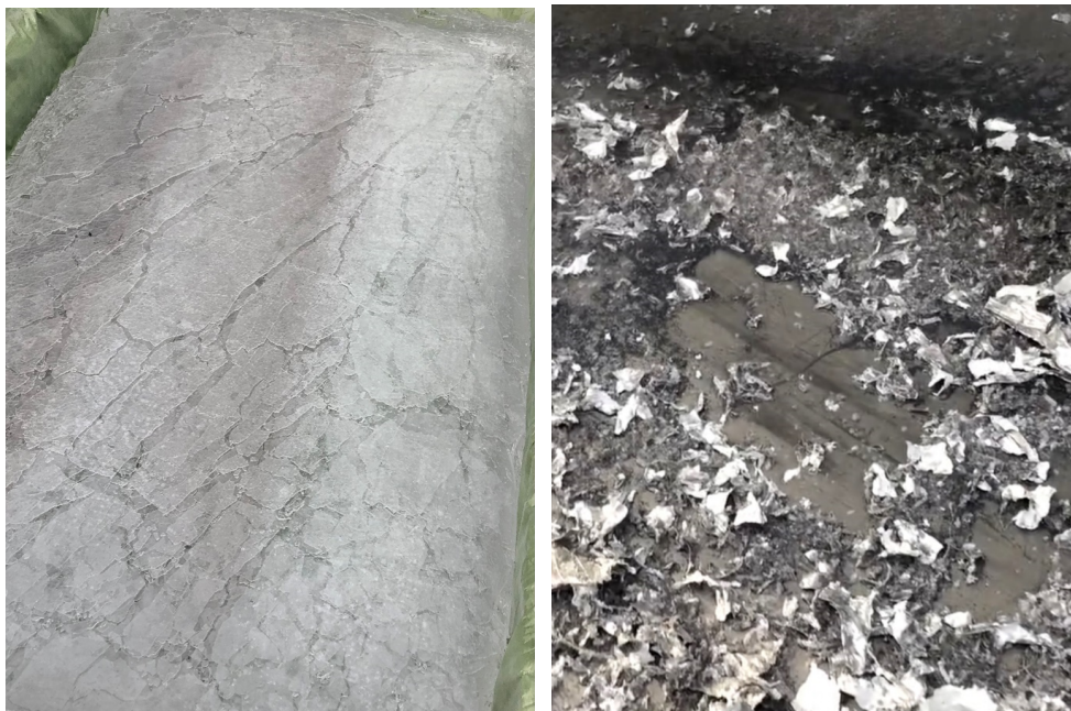
Figure 8: Clean glass cullet collected after water jet treatment (left) and separated polymer fraction with metal and solar cell fragments prior to further recycling (right) (Credit: LuxChemtech GmbH)
