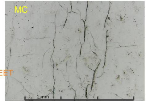
Crack filling (no voids)
