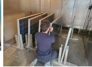
Test-case I : A **preventive maintenance coating process** was developed to stop the propagation of formed microcracks in weathered backsheets and to avoid the formation of deep backsheet cracks. The first test modules were coated in the field in June 2020 by (i) filling the surface near cracks of the BSs outer layer and (ii) additionally providing a full-deck barrier coating layer. First promising results on the long-term behaviour of the repair solutions exist after nearly 3 years now.
