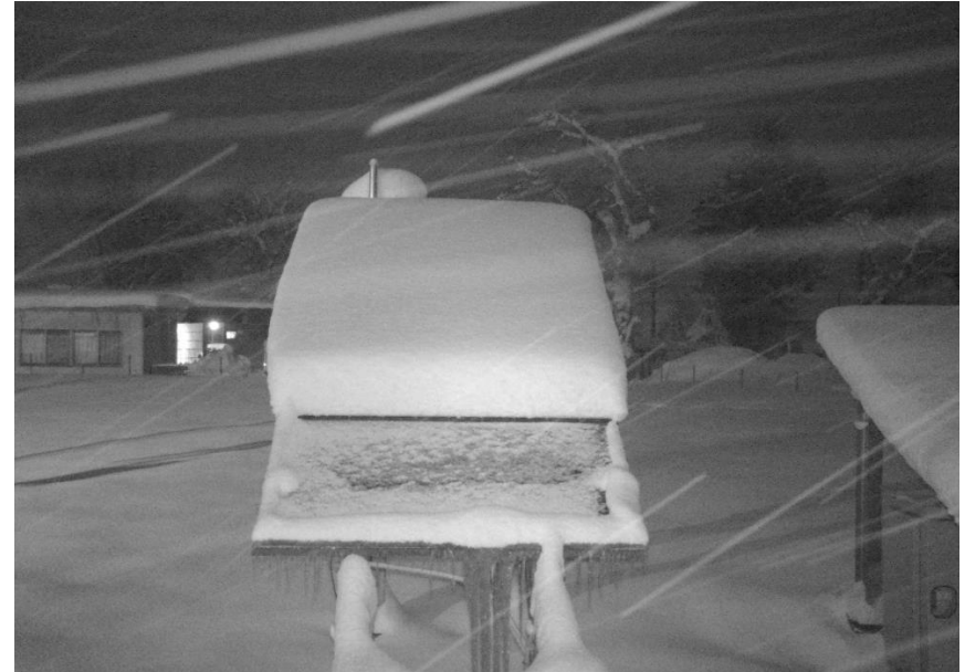
3-module sub-row with bottom module heated [AIST, Shinjo, JP]
