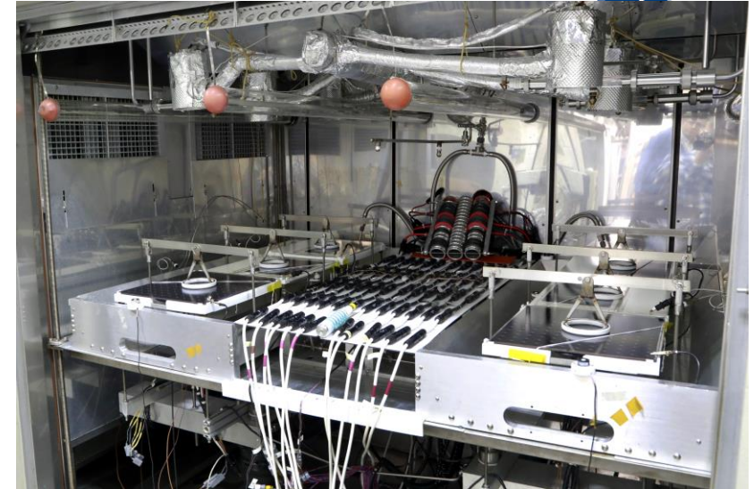
C-AST chamber, from the uncapped connector experiment; Source: David Miller, NREL..
