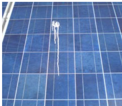
Figure 17: Shading due to dropping. Image from [31].
