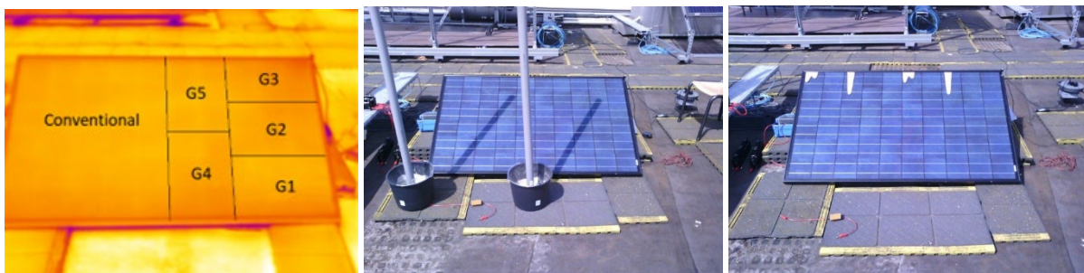
Figure 33: Cell sectors in the smart module, pole and bird droppings shading scenarios [53].
