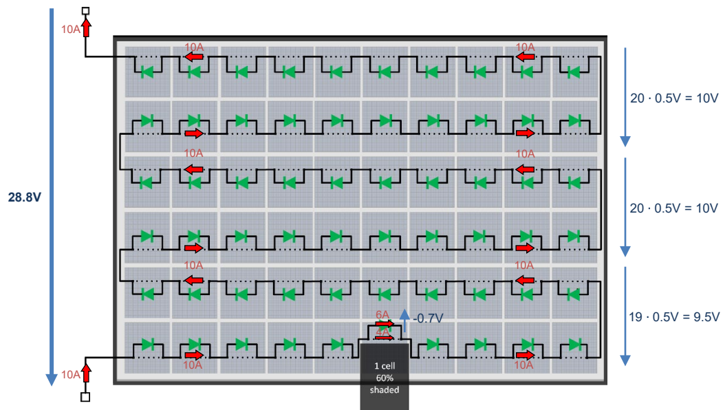
Figure 6: Internal circuitry of a hotspot-free PV module with a bypass diode (in green) installed at each PV cell [17]. For the case that one shingled solar strip is shaded by 60%, the ensuing current paths, as well as their magnitudes are visualised in red and the resulting voltages in blue (PV module voltage in bold letters).
