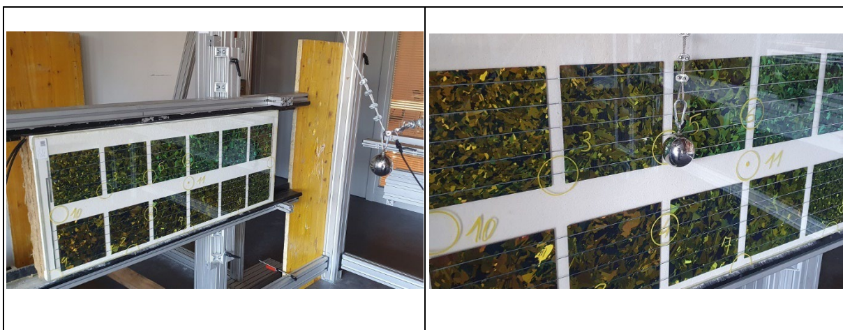
Figure 3.4 Hard body impact test equipment (left) and detail (right).
