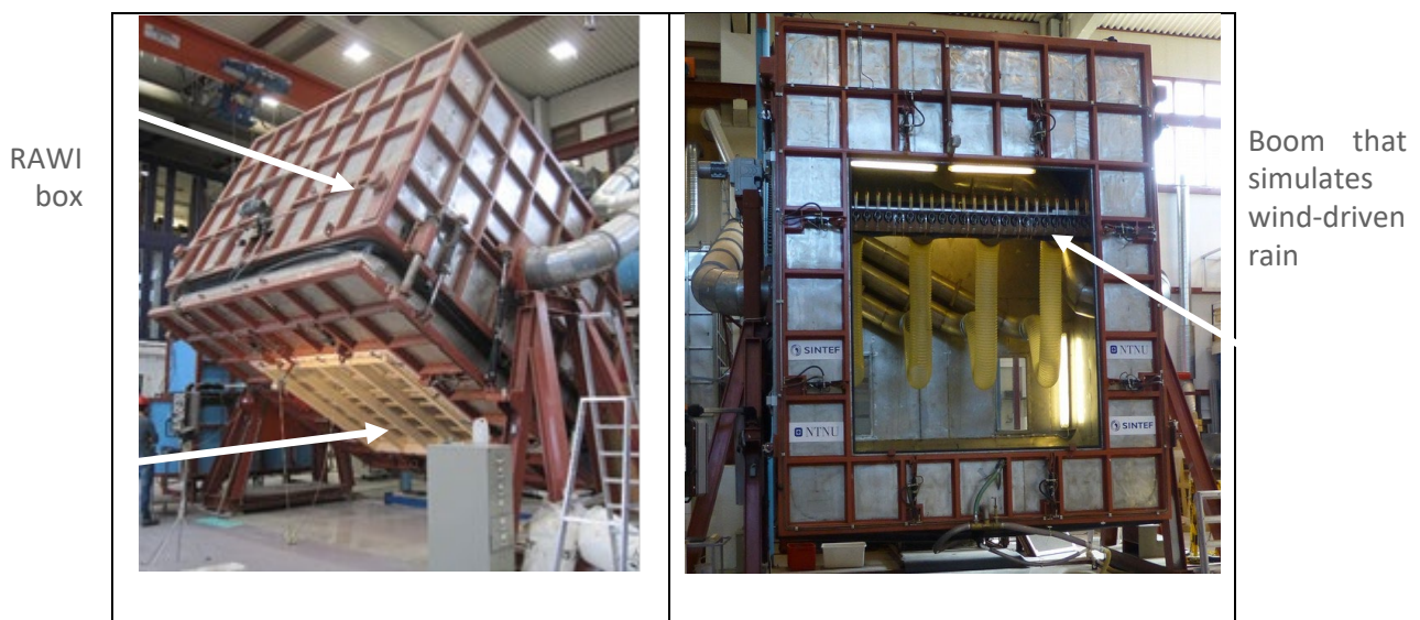
Figure 3.16 Large-scale rotatable box for rain and wind tightness testing of sloping building surfaces (RAWI box), while test is running (left) and RAWI box without a test sample (right) [57].
