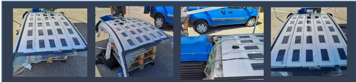
Figure 18: Exterior integration of irradiance test bench on vehicle roof.
