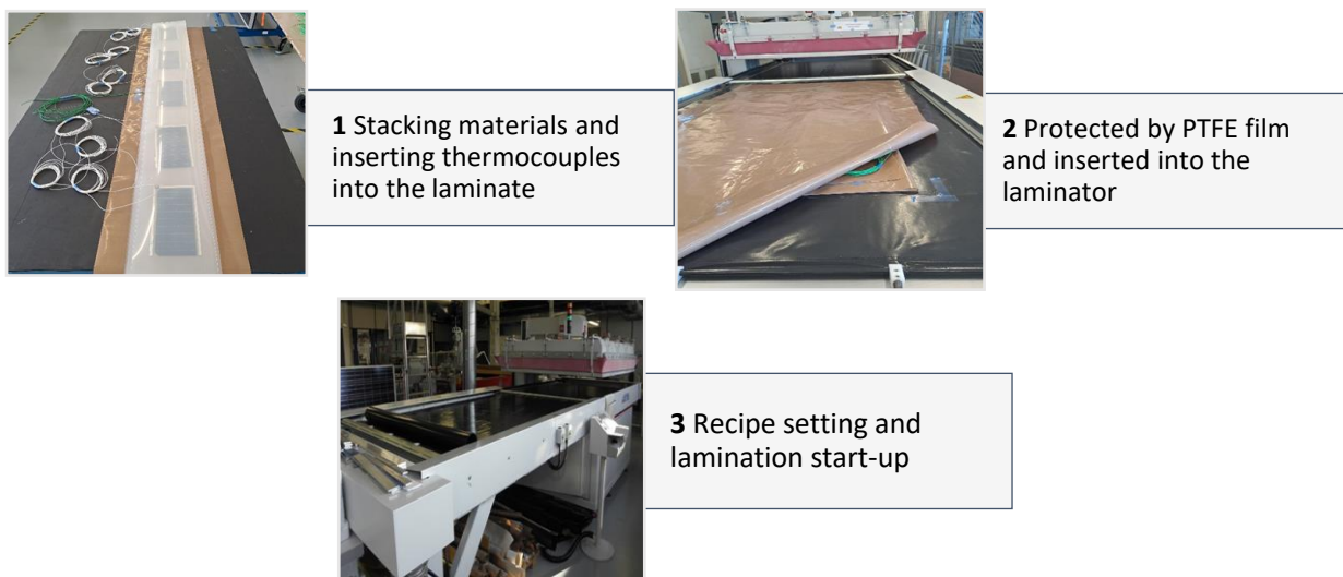
Figure 11: Assembly and introduction of cell strips into the laminator.
