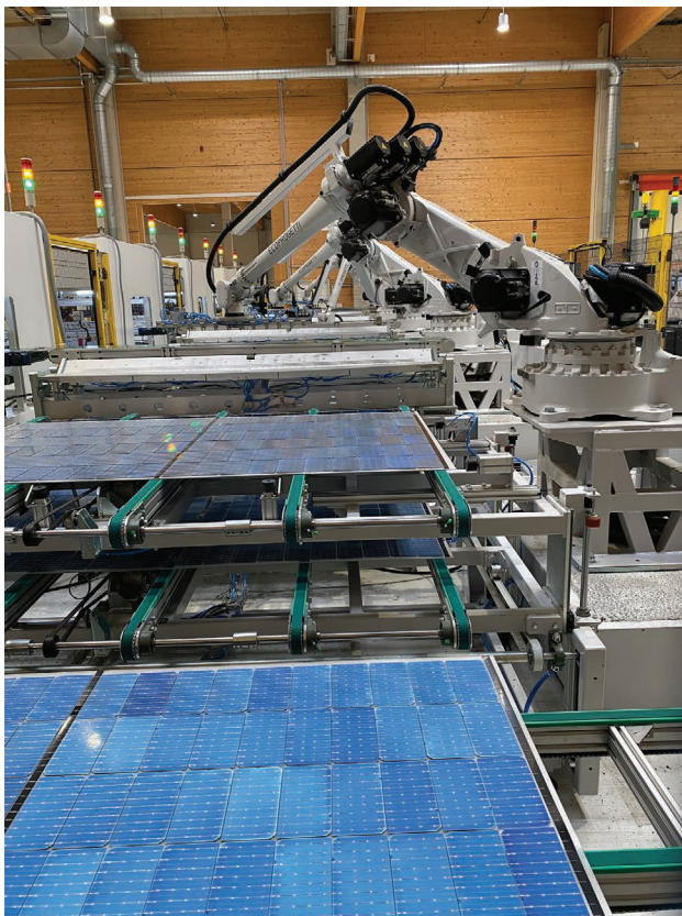
Figure 3.2 (from left to right and top to bottom): “Half-cut” crystalline silicon PV cells; PV cells prepared for stringing; preparation of the cell layout of the module; standard high-efficiency PV modules with backsheet foil (left), and with black backsheet foil for “all black” appearance (right). Photos taken at the Sonnenkraft GmbH facility in Austria (credits: Astrid Schneider, TU Wien).
