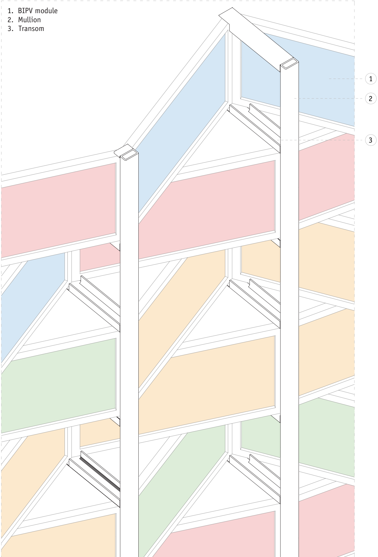
Figure 5.128 Gothenburg Garage. Axonometric drawing of the BIPV shading device. Credits: adapted by Ana Marcos Castro from Soltech Energy Sweden®.
