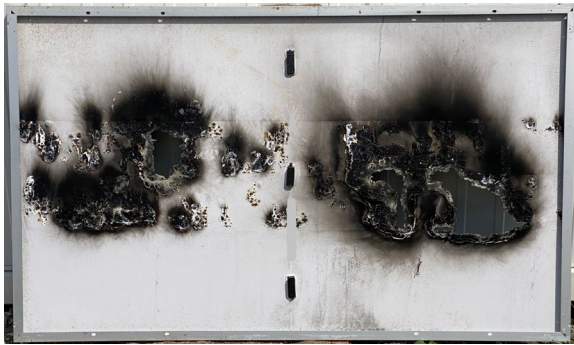
Figure 15: Rear side of TOPCon PV module with failure mode A being shaded by natural obstacles. Module has already been dismantled from the mounting rack.
