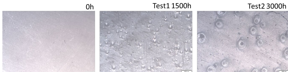
Figure 22: Detached surface of the PO encapsulant from the glass in the original state 0 hours and after two types of accelerated ageing tests. Test1: constant Xe-irradiation at 1000 W/m 2 at elevated temperature (chamber 65°C, PV module 96°C) and humidity (80%r.H.). Test2: sequential (i) 500 hours DH, (ii) 50 temperature cycles and (iii) 200 hours Xe-irradiation at 1000 W/m 2 , 3 sequences.
