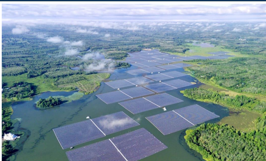
Photo 24: Aerial view of the largest floating solar in Malaysia located at Danau Tok Uban in the state of Kelantan. The solar plant has achieved its commercial operation date in January 2025 with total generation capacity of 60MWac.
