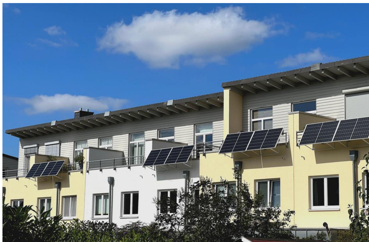
Photo 13: Balcony power plants in a terraced housing estate (© embeki – stock.adobe.com).
