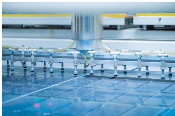
Photo 20: Bifacial cells string deposition after soldering. Photo courtesy of FuturaSun.
