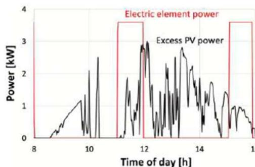
Figure 7. Electric element power (3.6 kW) compared to the available excess PV power when the water heating is only controlled by a tank thermostat (from [8]).
