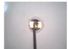
12. Supplying fluid soldering
