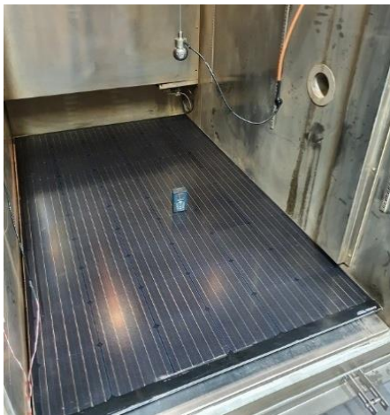
Source: SUPSI PVLab – Impact test in climatic room with different temperatures
